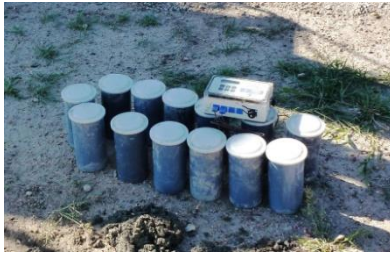
Figure 1. Cylinders cast from paving
