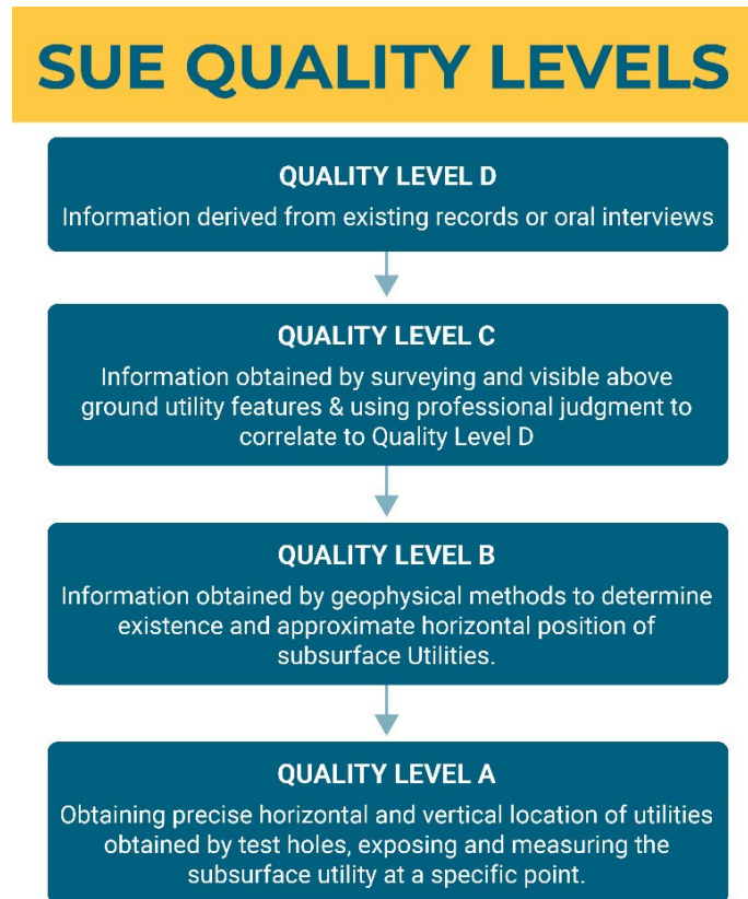
Figure 7-2. Subsurface Utility Engineering Quality Levels
