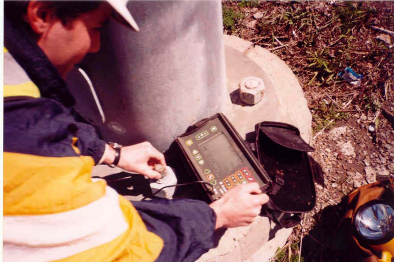
Figure 33. Ultrasonic Testing of Anchor Rods.
