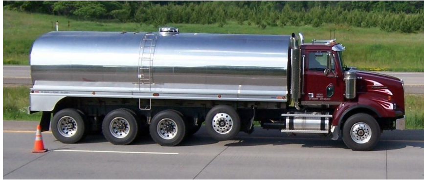
Figure 8. Photo. Class 7, single-unit truck with four of its five axles in contact with pavement.
