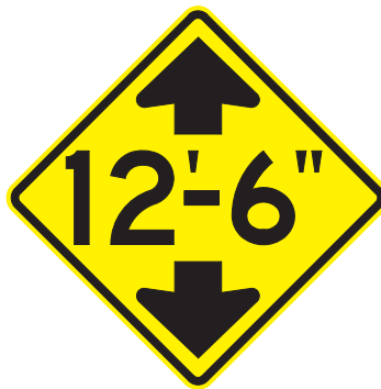
W12-2 Erected in advance of bridge
