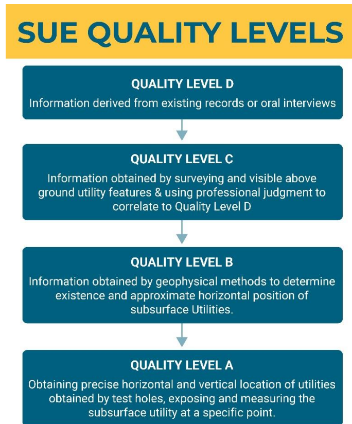
Figure 7-2. Subsurface Utility Engineering Quality Levels
