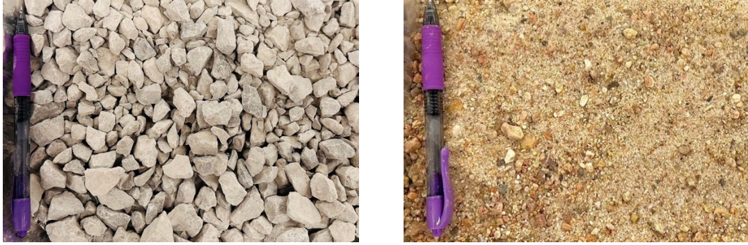
Figure 3.1 NA used in this study: a) Limestone (LS) and b) Sand and Gravel (SG).
