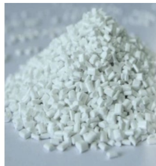
Figure 2.3 Granular UHMW Particles Obtained After Shredding ( Hongju, n.d.).
