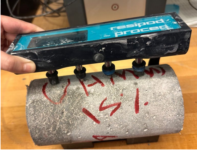
Figure 3.26 Test setup for surface resistivity of concrete.
