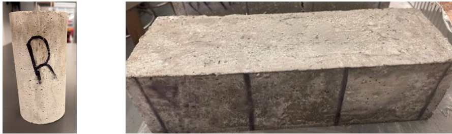
Figure 3.19 Concrete Samples a) 4 in. x 8 in. cylinder b) 6 in. x 6 in. x 20 in. beam.
