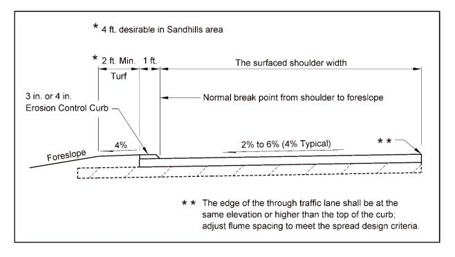
3-inch or 4-inch Erosion Control Curb
