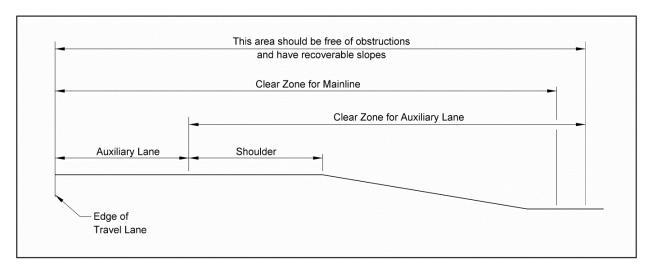
Note: Use the larger clear zone as measured from the edge of the travel lane or from the edge of the auxiliary lane.
