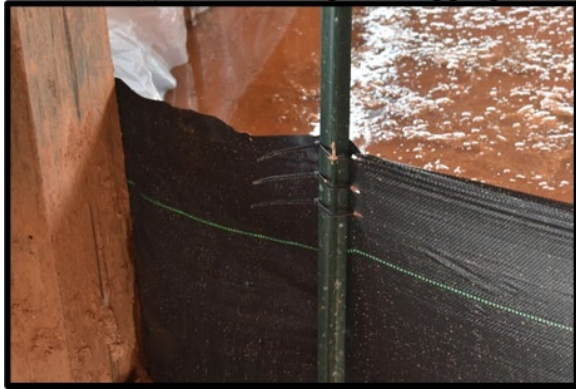
(c) stretching of fabric around zip-ties
