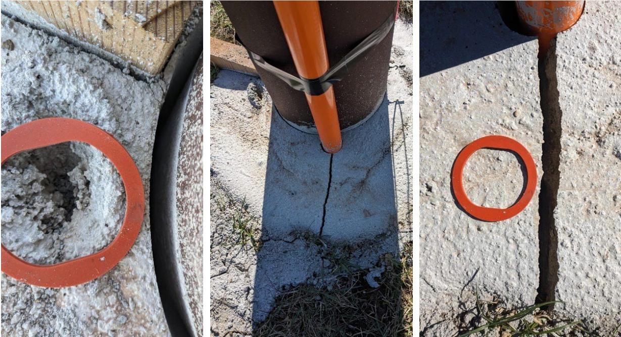
Figure 6.32 Observed damage in poles with concrete backfill after static tests
