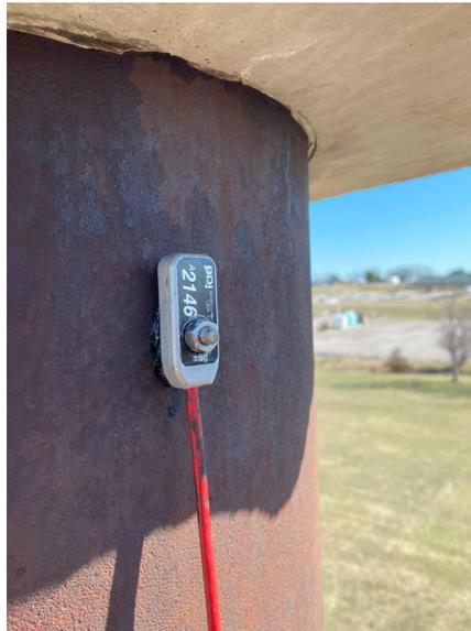
Figure 4.11 Accelerometers used to measure the acceleration at different locations during dynamic tests
