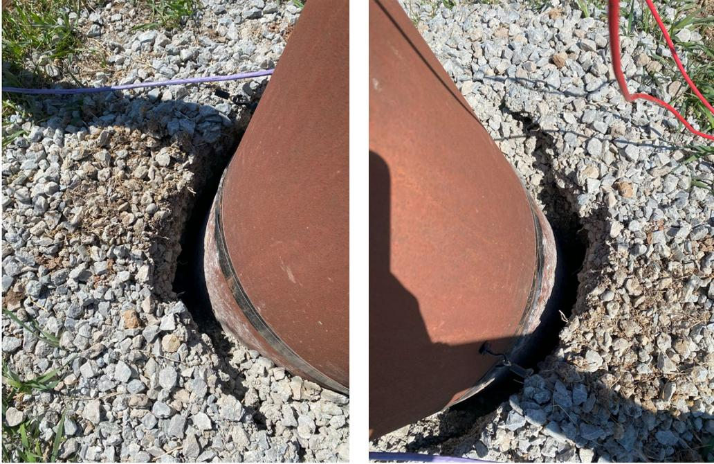
Figure 6.33 Observed damage in poles with gravel backfill after static tests
