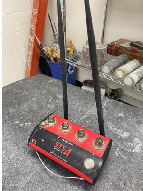
Figure 4.5 STS404 Wireless Intelliducer Node
