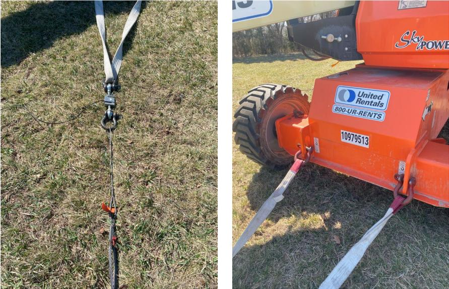
Figure 4.8 Pull setup for static and pluck tests
