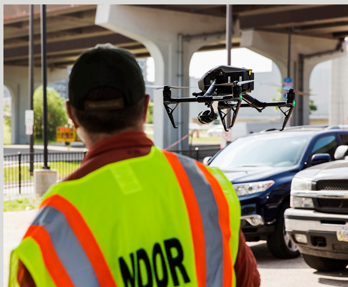
Drones are used to supplement visual inspections of bridges.
