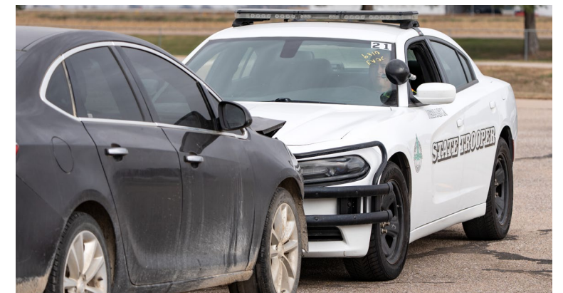
Pushing crashed vehicles opens lanes to traffic quickly and reduces roadway clearance times.
