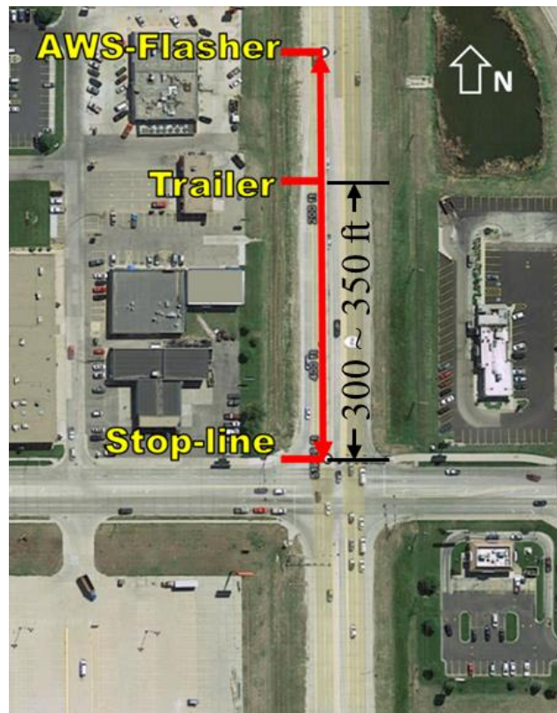
Figure 3.6 Trailer placement on the roadside of the approach at the study sites
