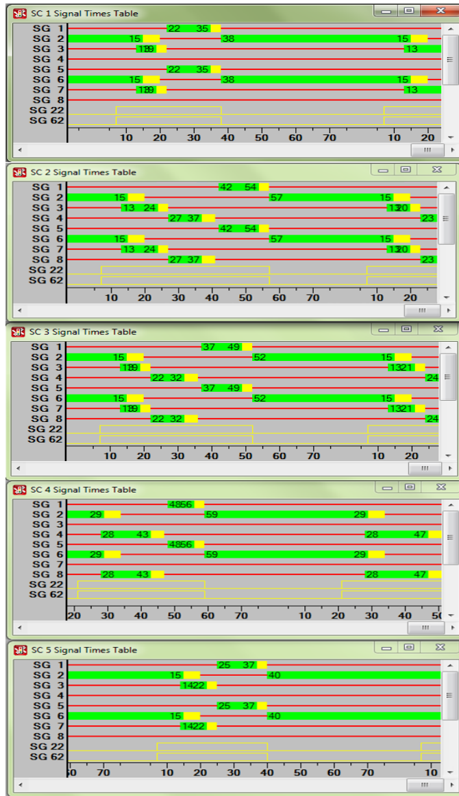
Figure 7.2 Actuated signal timing for the 5 coordinated intersections
