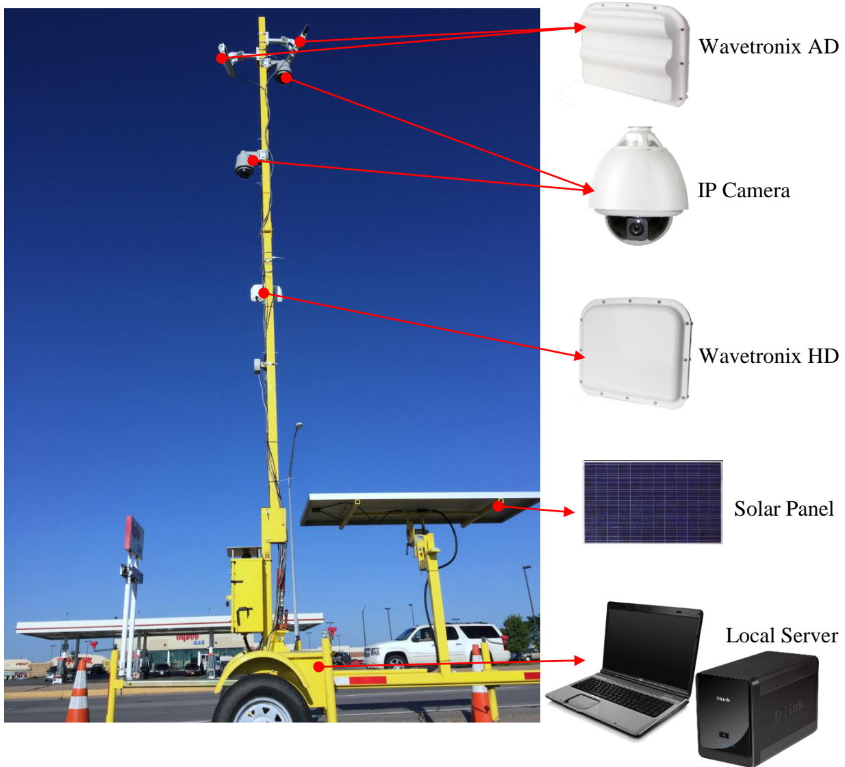
Figure 3.1 Mobile trailer data collection (MTDC) system
