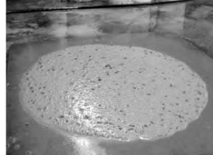
FIG. X1.3 VSI = 2 - Evidence of a Mortar Halo and Water Sheen.
