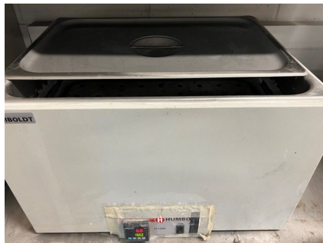
Figure 5.4 Hot bath for thermal treatment of selected specimens
