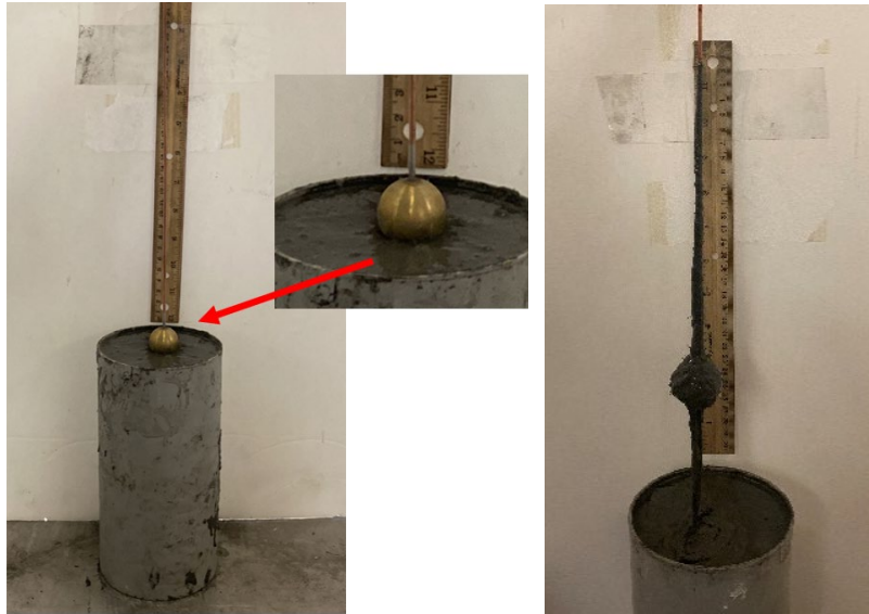
Figure 4.5 Falling-ball test set up (left: before ball settling; right: after ball settling)
