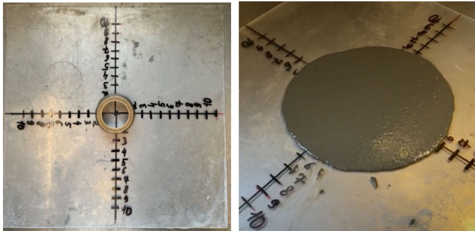
Figure 4.2 Flow and flow time test setup (left) and example of tests (right)
