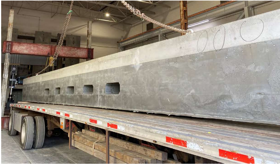
Box Beam with openings (Gage Brothers 2021)
