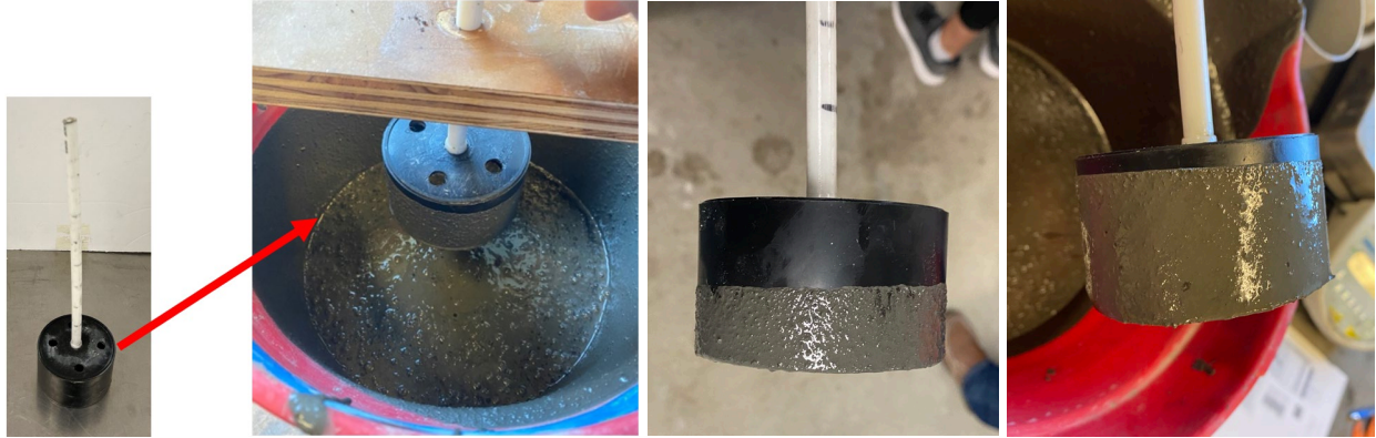
Figure 4.6 Penetration test setup and examples of results (left to right: test setup; mixture with medium penetration: and mixture with high penetration)
