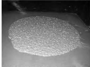
FIG. X1.1 VSI = 0 – Concrete Mass is Homogeneous and No Evidence of Bleeding.
