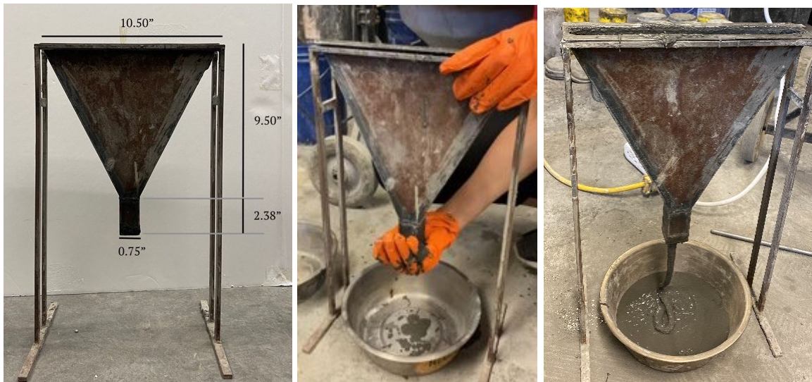
Figure 4.4 Mini V-funnel test set up (from left to right: test setup dimension; blocking of mini-V-funnel opening for mixture to settle; and UHPC mixture flowing out from the opening)
