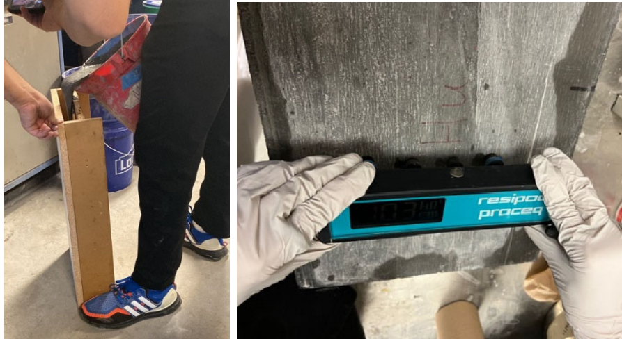
Figure 4.8 Segregation test specimen preparation and process (left: specimen casting; right: measure potential fiber segregation with resistivity meter)
