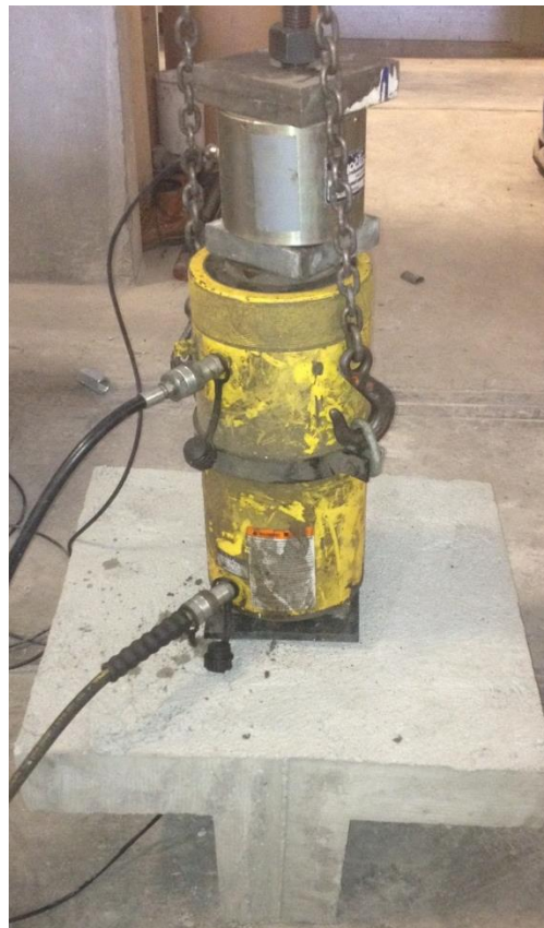
Figure 5.8: Pullout test setup of shallow T-girder specimens
