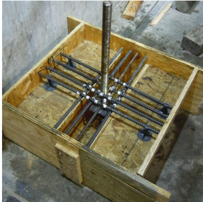
Figure 5.7: Forming and reinforcement of shallow T-girder specimens
