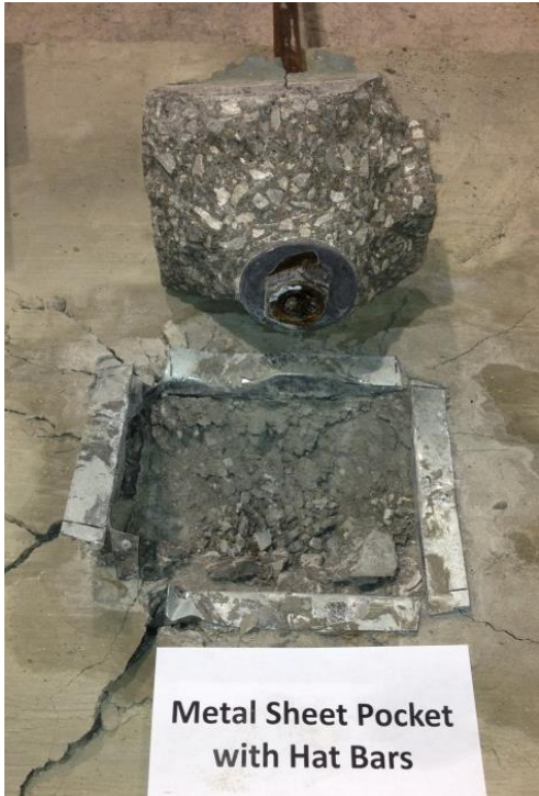
Figure 5.35: Pullout failure modes of the four pockets
