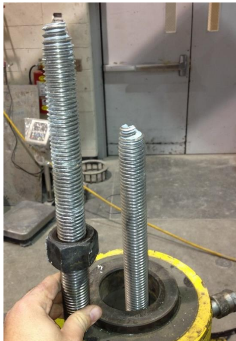
Figure 5.17: Rupture of the TR
