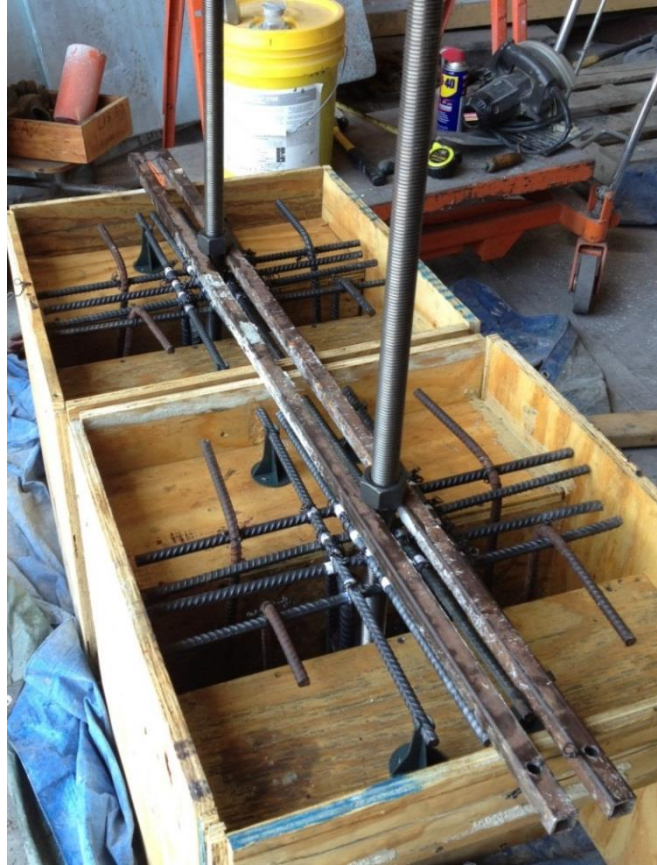
Figure 5.12: Forming and reinforcement of deep T-girder specimens
