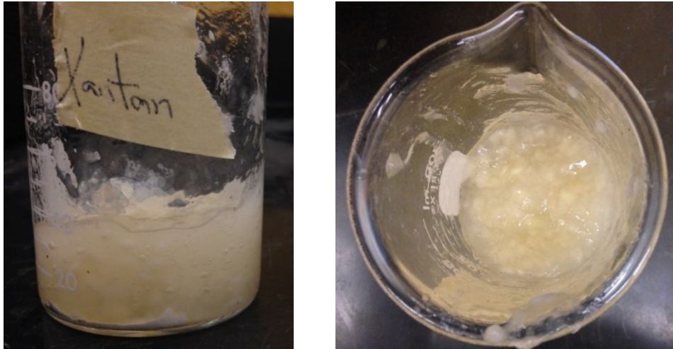
Figure 2.5 Solution of mixed 30 ml water and 2 gr Xanthan (Song et al., 2018)
