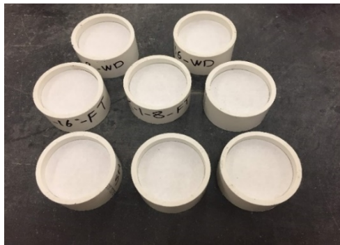
Figure 3.18 Preparing samples for weathering (Song et al., 2018)
