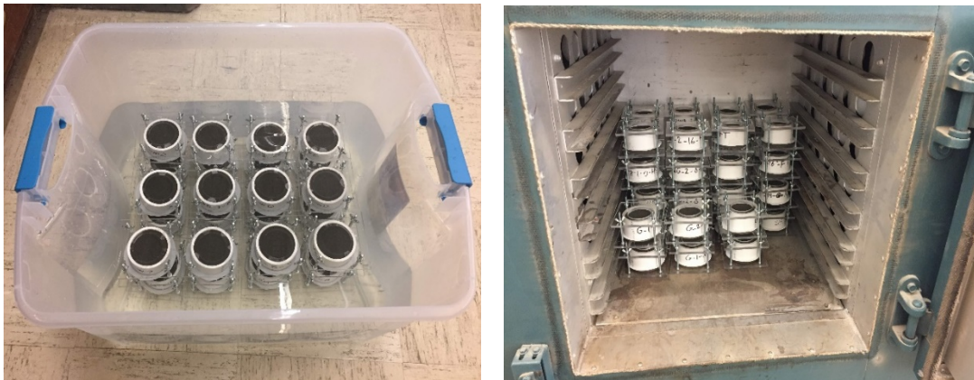
Figure 3.20 Water bath and oven used for wetting and drying soil samples, respectively
