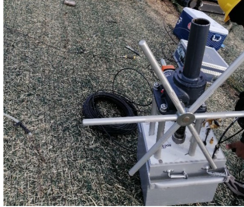
Figure 5.8 Scene of TEXAM pressuremeter deployed to the field
