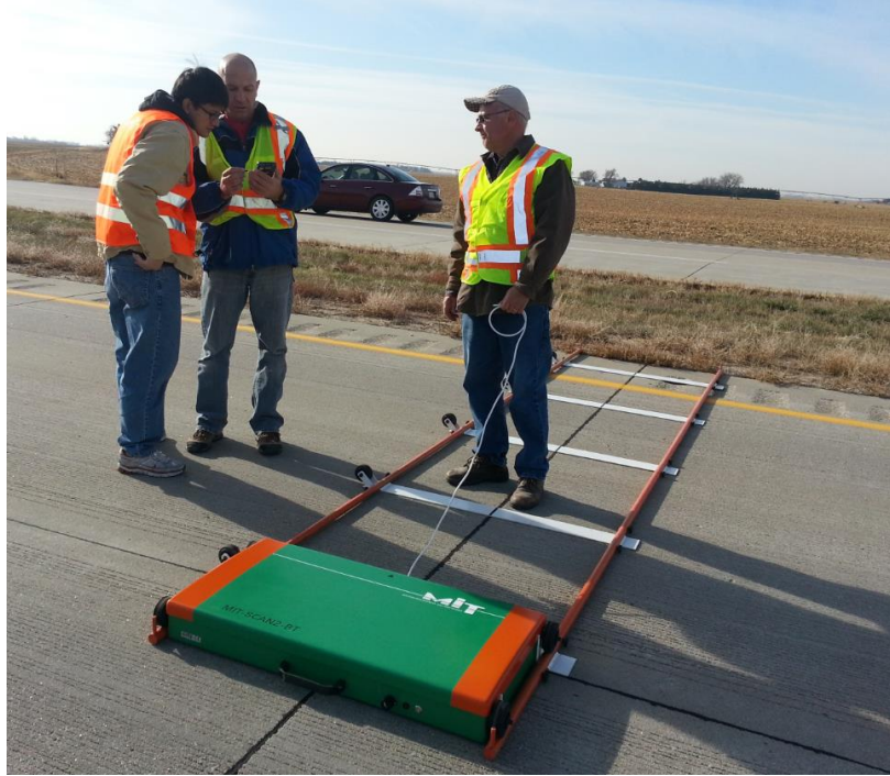
Figure 1.3 A joint being scanned by MIT Scan-2
