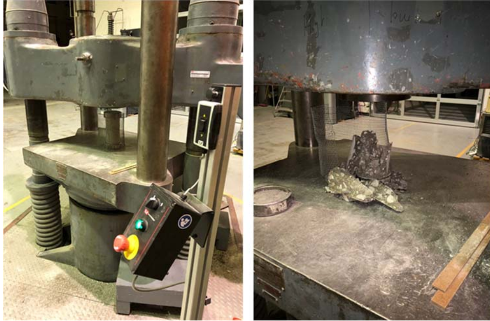
Figure 3-7. Compressive strength test setup
