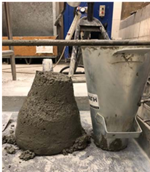
Figure 3-1. Slump test example
