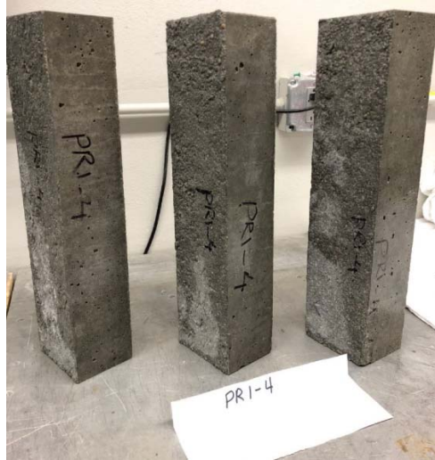
Figure 3-10 Wet/Dry specimens after 28 days of curing
