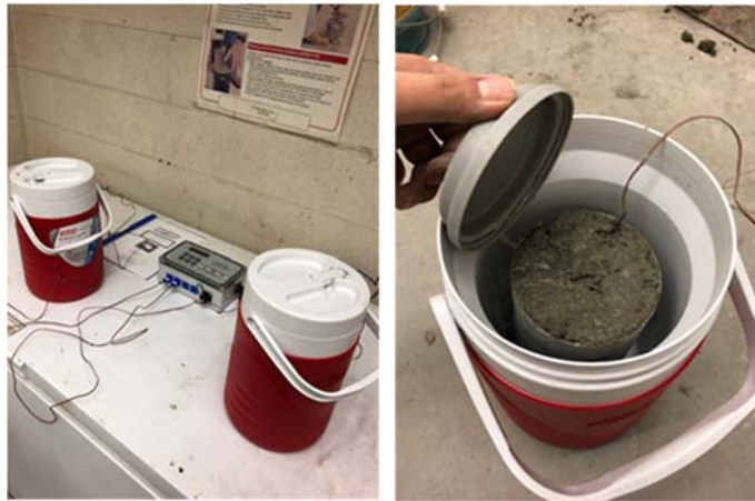
Figure 3-6. Maturity meter test setup
