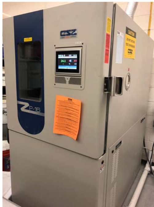
Figure 3-12. Environmental chamber for cold temperature simulation
