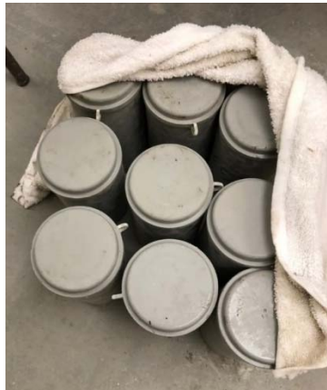
Figure 3-5. Testing cylinders for compressive strength test
