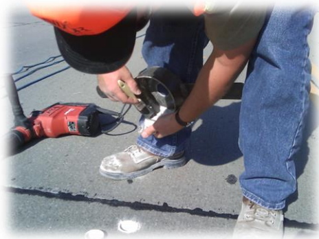
Figure 17. Drilled Dust Sample Collection
