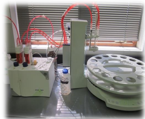
Figure 16. Chloride Ion Testing by Automatic Titrator
