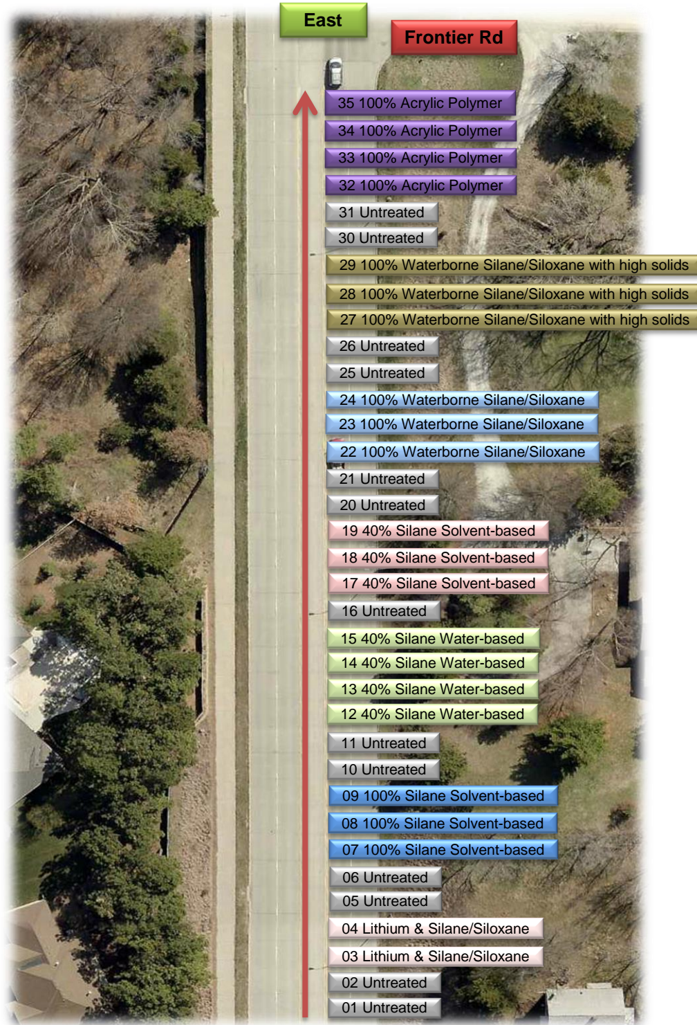
Figure 3. Layout of Sealer Test Panels Old Cheney between 62nd St and Frontier Rd
