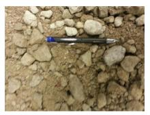
Figure 4 . Aggregate Sample for 40%RCA- 60% 47B Fine
