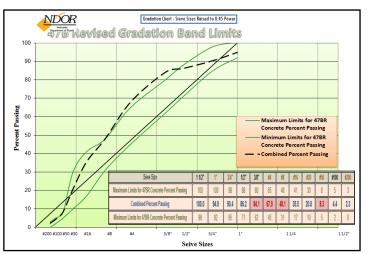
Figure 2. Combined Aggregate Gradations 40% RCA - 60% 47B Fine
