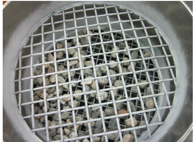
Figure 26. Aggregate Through a Series of Sieves
