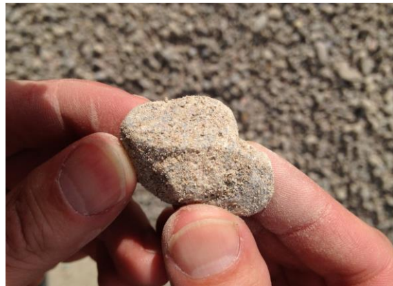
Figures 12 & 13. Aggregate Coating Dust
