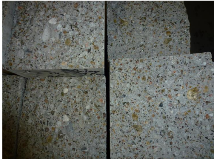
Figure 19. Flexure Strength Break Through Aggregate
