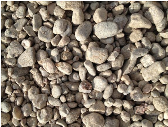
Figures 12 & 13. Aggregate Coating Dust
