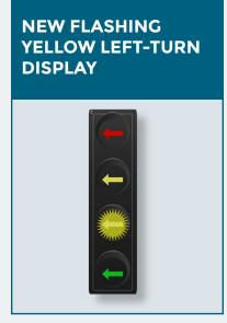
While you may be used to seeing the traditional left-turn traffic signal displays, NDOT has been implementing the new flashing yellow left-turn traffic signal displays because studies have shown that using them reduces left-turn crashes at intersections.
