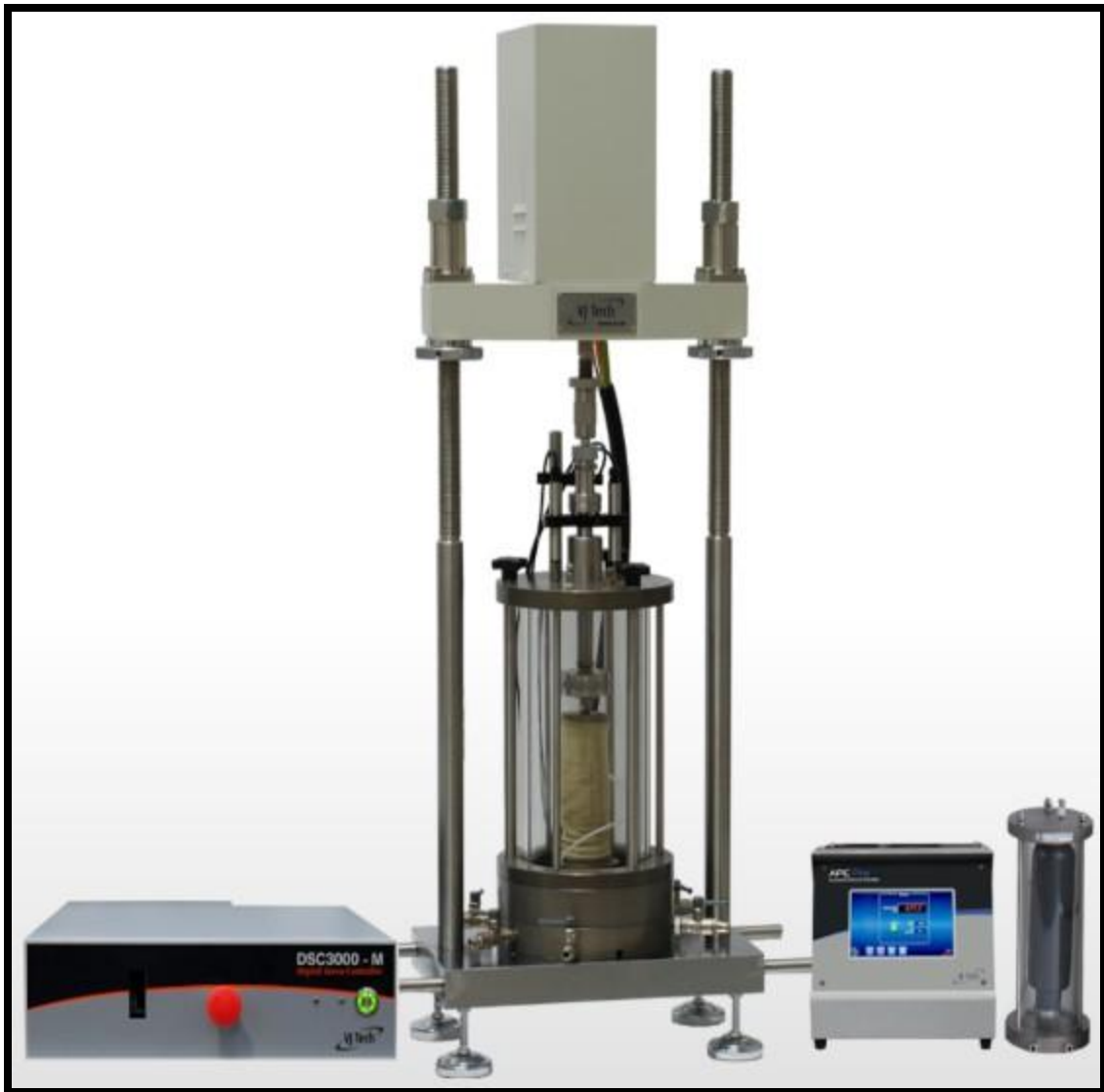
Figure 5.4-3 – Resilient Modulus System (VJ Tech Limited)
