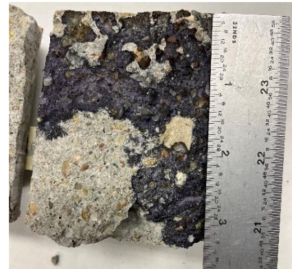
Figure 3- The control section core after sealer was applied.
