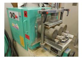
Figure 1. End Grinding Equipment
