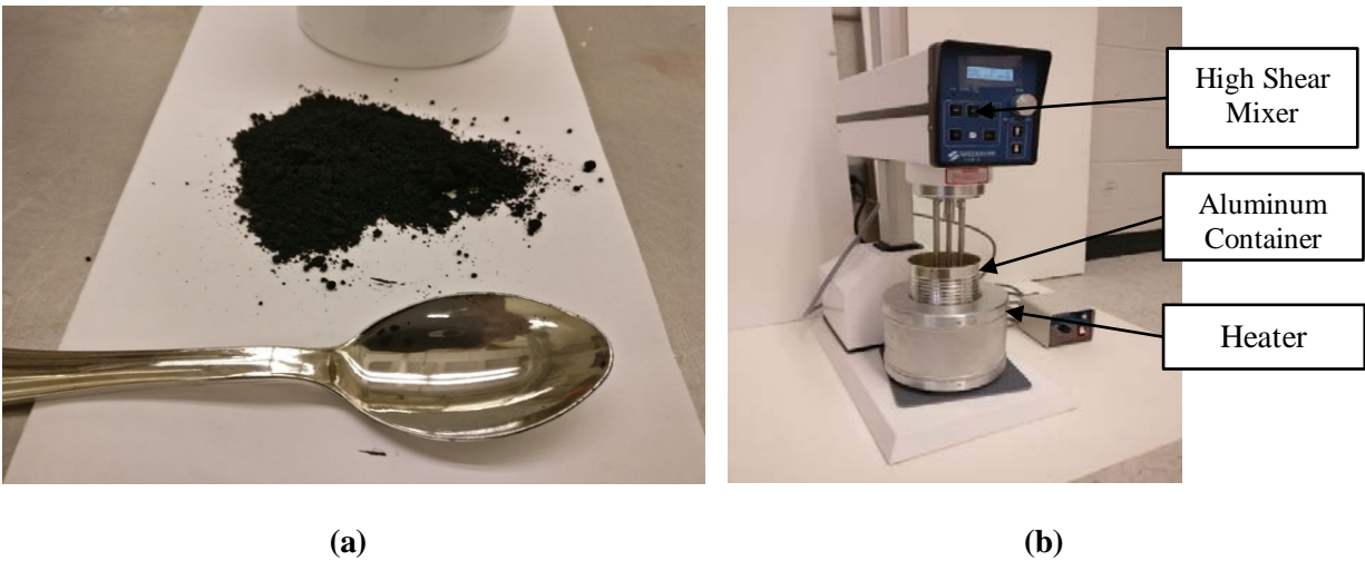
Figure 12: Nano-filler and mixing method: (a) nanostructured graphite-250 that was used in the preliminary investigation, (b) Silverson high shear mixer with the aluminum container and heater.
