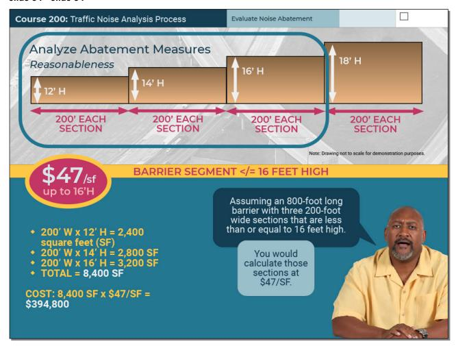
For example, assuming you have an eight-hundred-foot long barrier with three two-hundred-foot wide sections that are less than or equal to sixteen feet high. You would calculate those sections at forty-seven dollars per square foot.
