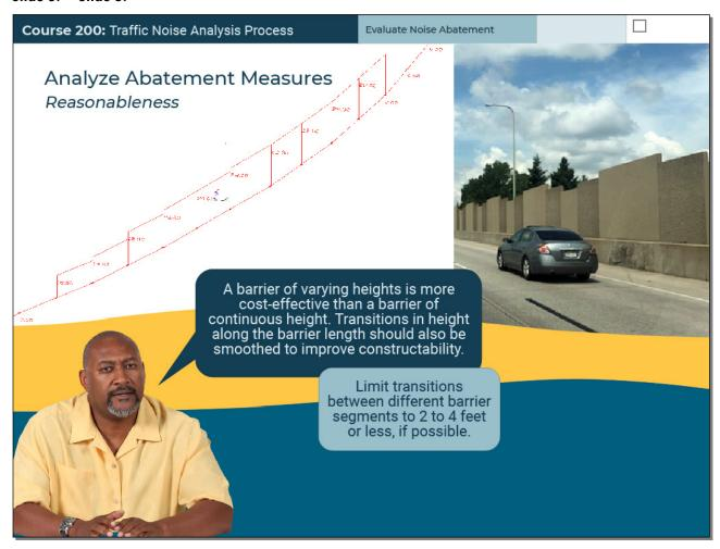
A barrier of varying heights is more cost-effective than a barrier of continuous height. Transitions in height along the barrier length should also be smoothed to improve constructability. Limit transitions between different barrier segments to two to four feet or less, if possible.
