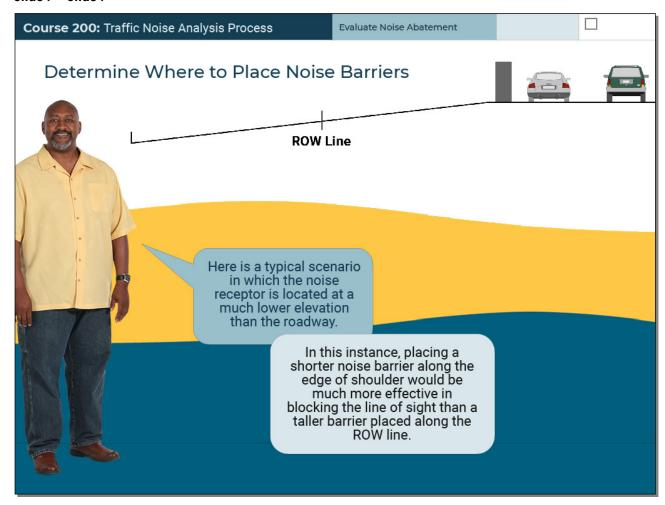
Here is a typical scenario in which the noise receptor is located at a much lower elevation than the roadway. In this instance, placing a shorter noise barrier along the edge of the shoulder would be much more effective in blocking the line of sight than a taller barrier placed along the right-of-way line.
