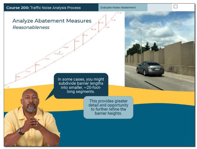
In some cases, and in coordination with the N-dot Noise P-Q-S, you might subdivide barrier lengths into smaller, approximately twenty-foot-long segments. This provides greater detail and opportunity to further refine the barrier heights.
