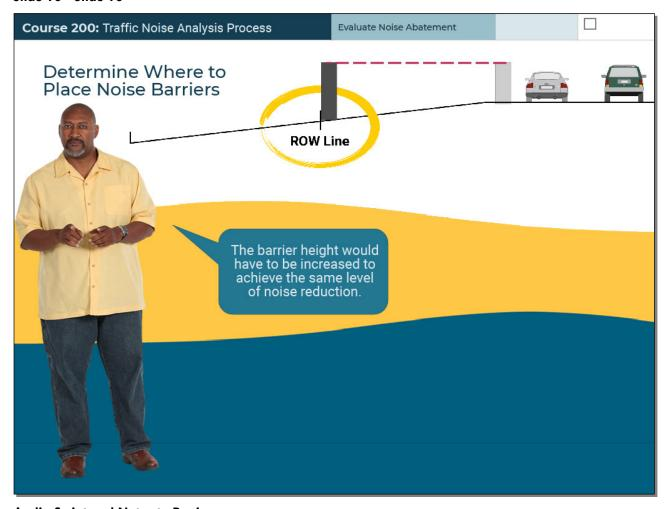
That's because the barrier height would have to be increased to achieve the same level of noise reduction.
