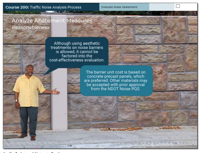
Although using aesthetic treatments on noise barriers is allowed, it cannot be factored into the cost-effectiveness evaluation. The barrier unit cost is based on concrete precast panels, which are preferred. Other materials may be accepted with prior approval from the N-dot Noise P-Q-S.
