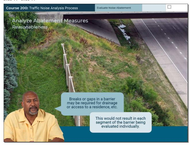
Breaks or gaps in a barrier may be required for drainage or access to a residence, etcetera. This would not result in each segment of the barrier being evaluated individually.
