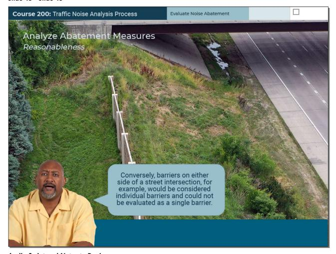
Conversely, barriers on either side of a street intersection, for example, would be considered individual barriers and could not be evaluated as a single barrier.
