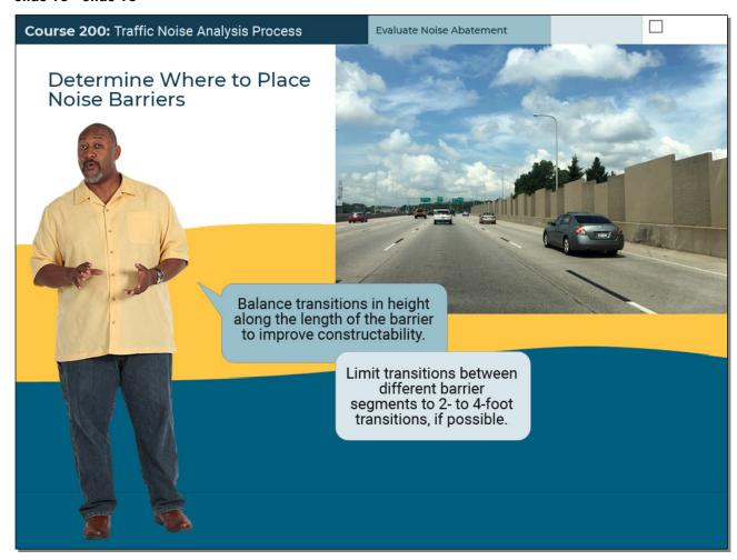
Balance transitions in height along the length of the barrier to improve constructability. Limit transitions between different barrier segments to two- to four-foot transitions, if possible.
