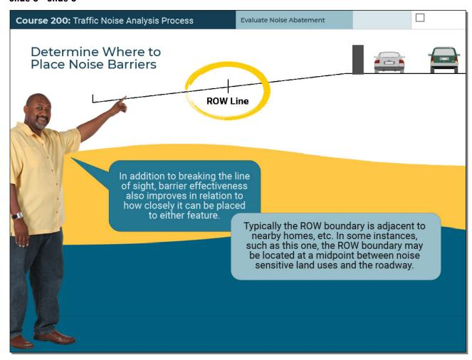
In addition to breaking the line of sight, barrier effectiveness also improves in relation to how closely it can be placed to either feature. Typically the right-of-way boundary is adjacent to nearby homes, etcetera. In some instances, such as this one, the right-of-way boundary may be located at a midpoint between noise sensitive land uses and the roadway.
