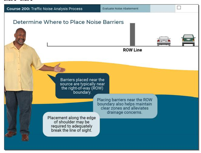
Barriers placed near the source -- meaning, the roadway -- are typically near the right-of-way boundary. Placing barriers near the right-of-way boundary also helps maintain clear zones and alleviates drainage concerns. However, in some instances, placement along the edge of shoulder may be required to adequately break the line of sight.
