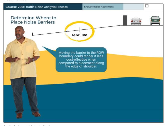
Moving the barrier to the right-of-way boundary could render it less cost-effective when compared to placement along the edge of shoulder.
