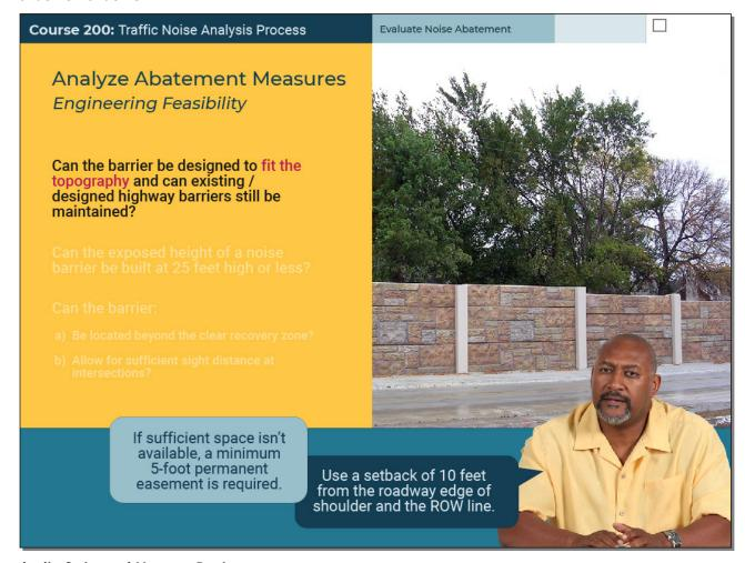
Use a setback distance of ten feet from both the roadway edge of shoulder, as well as the right-of-way line, if space allows. This allows for barrier repair and maintenance, such as mowing. However, if sufficient space isn't available, a minimum five-foot permanent easement is required.
