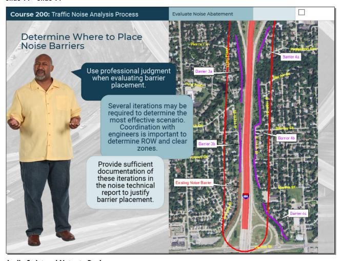
Use professional judgment when evaluating barrier placement. Several iterations may be required to determine the most effective scenario. Coordination with engineers is important to determine right-of-way and clear zones. Provide sufficient documentation of these iterations in the noise technical report to justify barrier placement.
