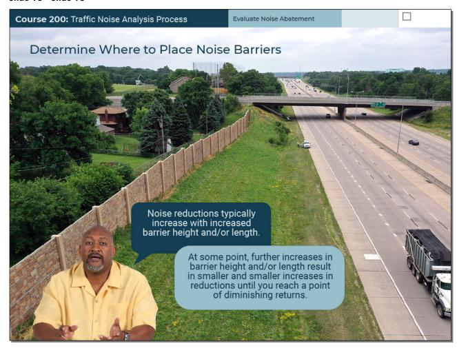
Noise reductions typically increase with increased barrier height and/or length. However, at some point, further increases in barrier height and-or length result in smaller and smaller increases in reductions until you reach a point of diminishing returns.
