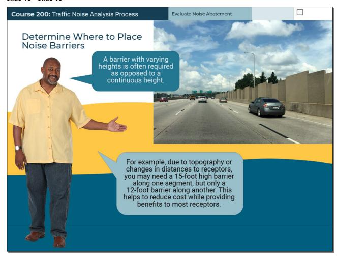
To achieve the most cost-effective results, a barrier with varying heights is often required as opposed to a continuous height. For example, due to topography or changes in distances to receptors, you may need a fifteen-foot high barrier along one segment, but only a twelve-foot barrier along another. This helps to reduce cost while providing benefits to most receptors.
