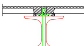
PC I Beam + UHPC Ribbed Slab
