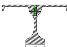
UHPC I Beam + UHPC Ribbed Slab
