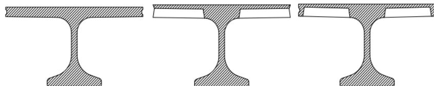
UHPC DIB with Solid Slab
