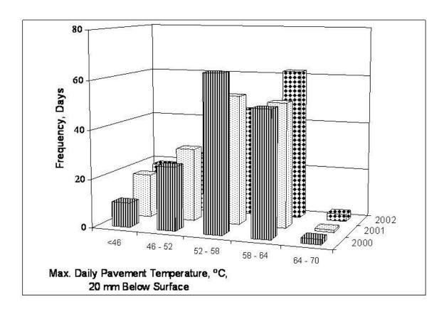
FIGURE 3 Frequency of Maximum Daily Pavement Temperature, Highway-56.
