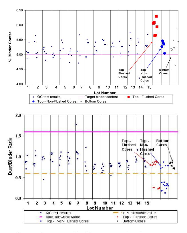
FIGURE 4 Comparisons of QA/QC Data with Field Cores for Highway-56.
