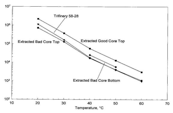
FIGURE 2 Comparisons of Extracted Cores and Original Asphalt by WRI (5).
