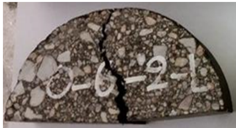
Figure 11. Off-center crack initiation for notch-less SCB specimens.
