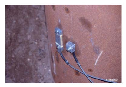
Figure 2.6: Accelerometer and strain gauge attached to the pile head
