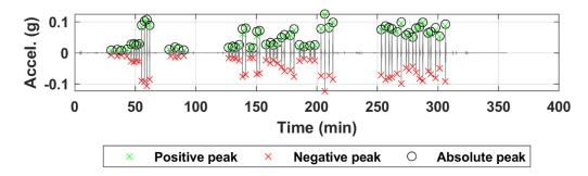
Figure B.249. Acceleration time history of sensor N16 for all truck passes at the NOBL West Yutan bridge structure.
