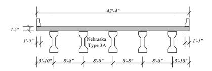
Figure 5.2. Schematic cross-section of the bridge.
