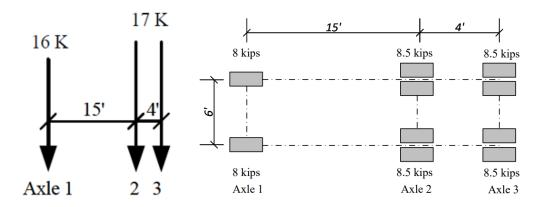
Figure C.380. NE Type 3 truck configuration.
