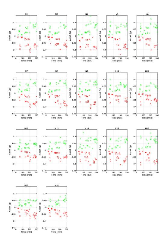
Figure B.233. Maximum acceleration values for each truck pass at the NOBL West Yutan bridge structure.
