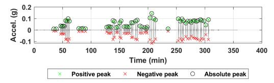
Figure B.237. Acceleration time history of sensor N04 for all truck passes at the NOBL West Yutan bridge structure.
