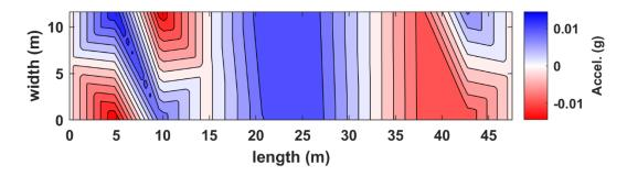
Figure B.47. Interpolated acceleration in plan view for truck pass 57 at the NOBL North bridge structure.
