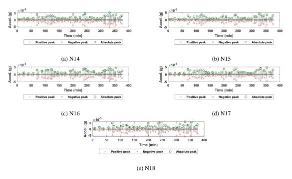
Figure 4.8. Acceleration time histories of the girder sensors for all truck passes at NOBL North.
