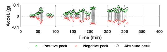
Figure B.251. Acceleration time history of sensor N18 for all truck passes at the NOBL West Yutan bridge structure.
