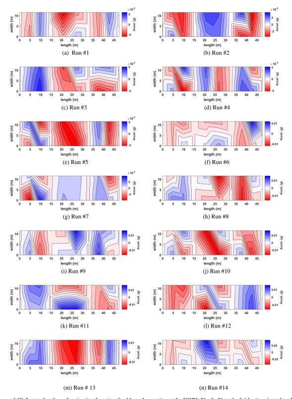
Figure 4.10. Interpolated acceleration in plan view for 14 trucks passing at the NOBL North. Note the bridge is oriented to the north direction (up on the page is north).
