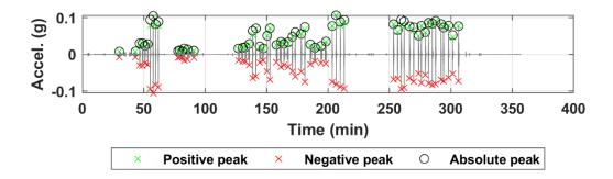
Figure B.253. Acceleration time history of sensor N20 for all truck passes at the NOBL West Yutan bridge structure.
