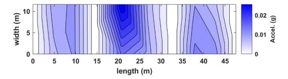
Figure B.64. Interpolated absolute-valued acceleration in plan view for truck pass 31 at the NOBL North bridge structure.
