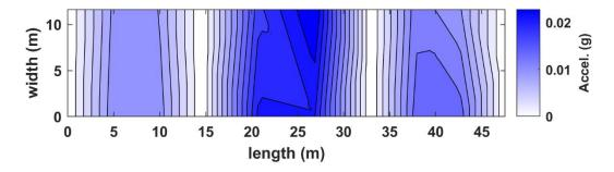
Figure B.69. Interpolated absolute-valued acceleration in plan view for truck pass 36 at the NOBL North bridge structure.
