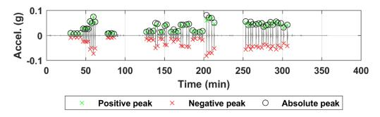
Figure B.245. Acceleration time history of sensor N12 for all truck passes at the NOBL West Yutan bridge structure.
