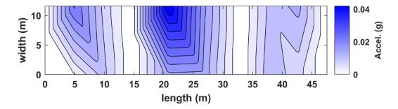
Figure B.85. Interpolated absolute-valued acceleration in plan view for truck pass 52 at the NOBL North bridge structure.
