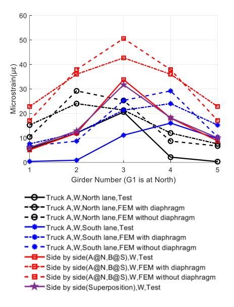
Figure C.402. Positive strain at 0.4 L of east end span, side-by-side loading, west direction loading.
