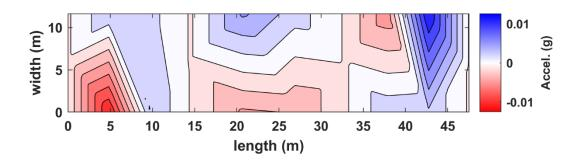
Figure B.17. Interpolated acceleration in plan view for truck pass 27 at the NOBL North bridge structure.
