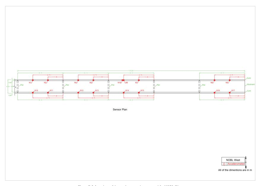
Figure B.3. Locations of the accelerometer instrumented for NOBL West
