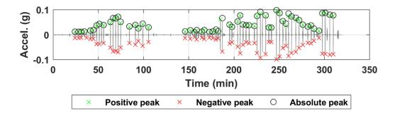
Figure B.105. Acceleration time history of sensor N14 for all truck passes at the NOBL East Yutan bridge structure.
