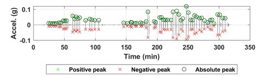
Figure B.101. Acceleration time history of sensor N10 for all truck passes at the NOBL East Yutan bridge structure.
