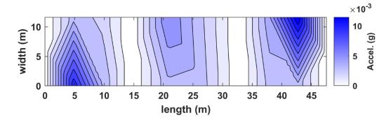
Figure B.60. Interpolated absolute-valued acceleration in plan view for truck pass 27 at the NOBL North bridge structure.
