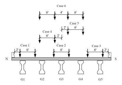
Figure 5.7. Transverse locations of trucks on the bridge.
