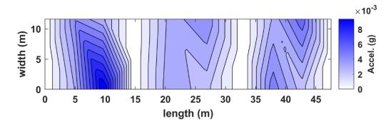
Figure B.77. Interpolated absolute-valued acceleration in plan view for truck pass 44 at the NOBL North bridge structure.
