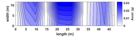
Figure B.84. Interpolated absolute-valued acceleration in plan view for truck pass 51 at the NOBL North bridge structure.
