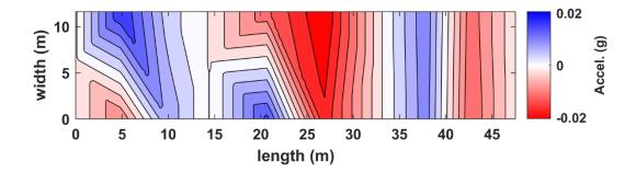
Figure B.25. Interpolated acceleration in plan view for truck pass 35 at the NOBL North bridge structure.
