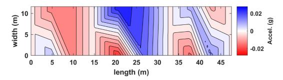
Figure B.27. Interpolated acceleration in plan view for truck pass 37 at the NOBL North bridge structure.
