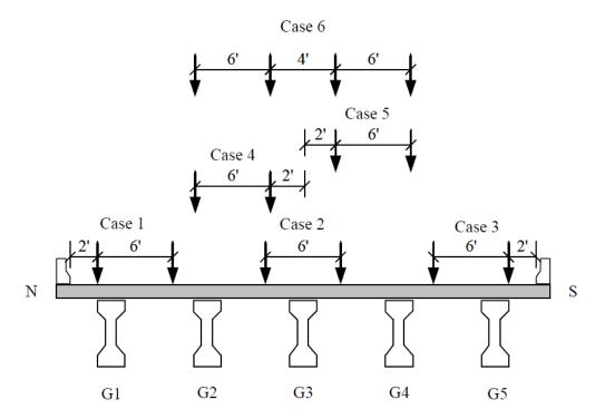
Figure C.381. Transverse locations of trucks on the bridge.
