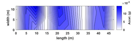
Figure B.66. Interpolated absolute-valued acceleration in plan view for truck pass 33 at the NOBL North bridge structure.
