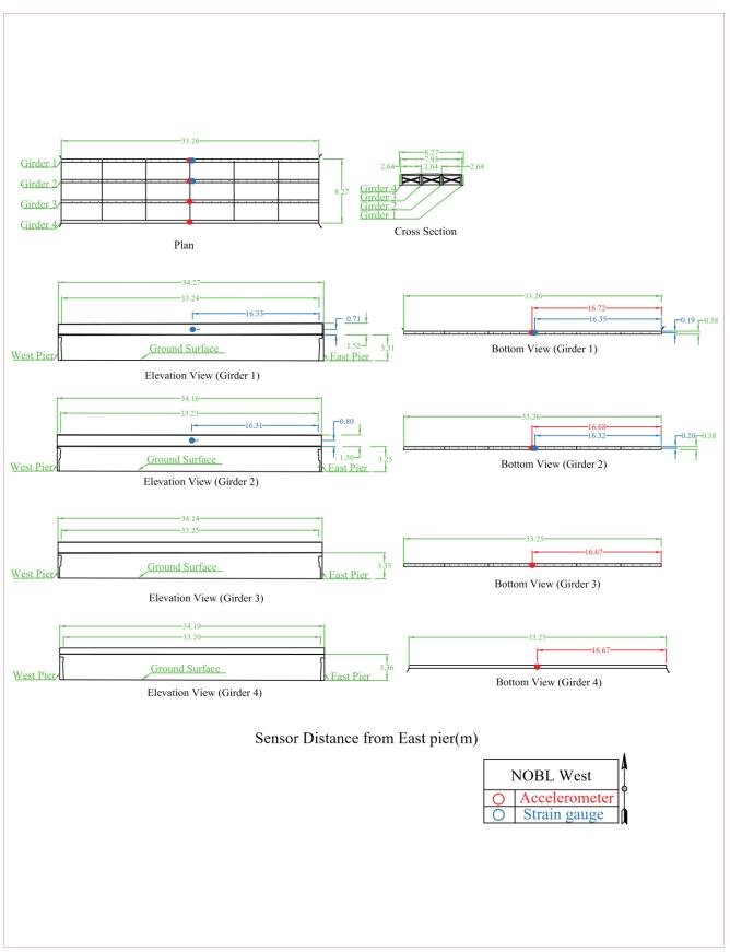
Figure B.4. Locations of the accelerometers instrumented to girders for NOBL West
