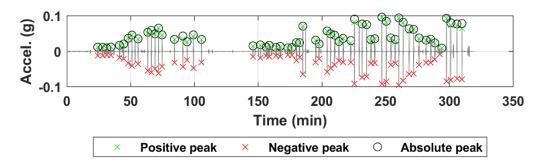
Figure B.97. Acceleration time history of sensor N06 for all truck passes at the NOBL East Yutan bridge structure.
