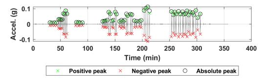
Figure B.242. Acceleration time history of sensor N09 for all truck passes at the NOBL West Yutan bridge structure.
