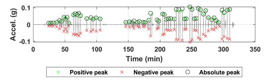
Figure B.103. Acceleration time history of sensor N12 for all truck passes at the NOBL East Yutan bridge structure.
