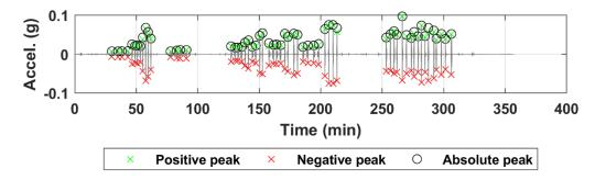
Figure B.255. Acceleration time history of sensor N22 for all truck passes at the NOBL West Yutan bridge structure.
