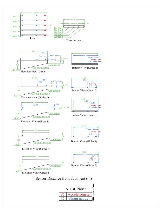
Figure 4.4. Locations of the accelerometers instrumented to girders for NOBL North.
