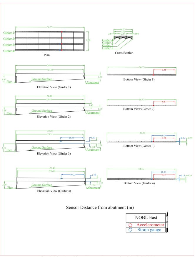
Figure B.2. Locations of the accelerometers instrumented to girders for NOBL East
