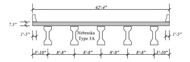
Figure C.375. Schematic cross section of the bridge.
