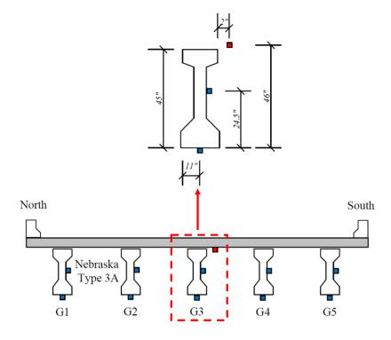
Figure C.377. Strain transducers installation locations in the bridge cross-section
