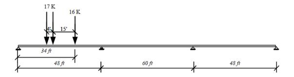
Figure C.391. Critical truck position for 0.4L of the end span.
