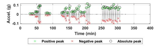
Figure B.252. Acceleration time history of sensor N19 for all truck passes at the NOBL West Yutan bridge structure.
