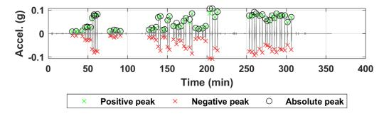
Figure B.248. Acceleration time history of sensor N15 for all truck passes at the NOBL West Yutan bridge structure.
