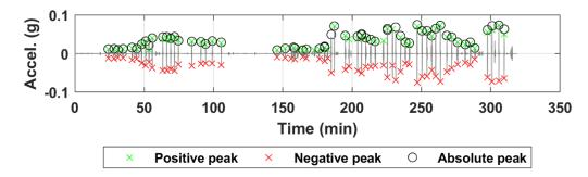
Figure B.107. Acceleration time history of sensor N16 for all truck passes at the NOBL East Yutan bridge structure.
