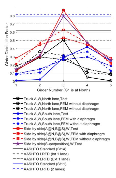
Figure C.403. GDF from positive strain at 0.4 L of east end span, side-by-side loading, west direction loading.
