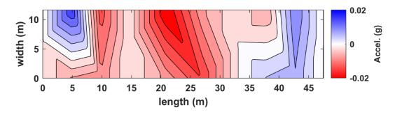
Figure B.45. Interpolated acceleration in plan view for truck pass 55 at the NOBL North bridge structure.
