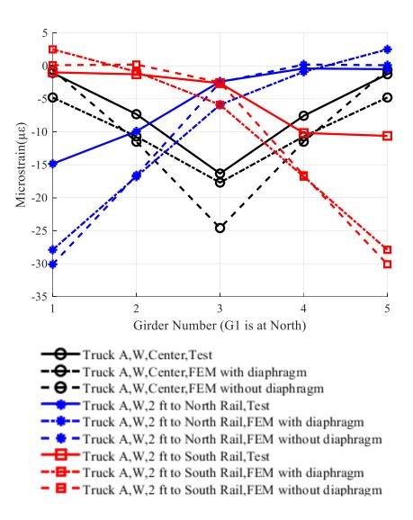
Figure C.400. Negative strain near east side of pier, west direction loading.
