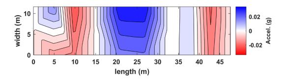
Figure B.41. Interpolated acceleration in plan view for truck pass 51 at the NOBL North bridge structure.
