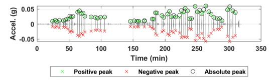
Figure B.110. Acceleration time history of sensor N19 for all truck passes at the NOBL East Yutan bridge structure.
