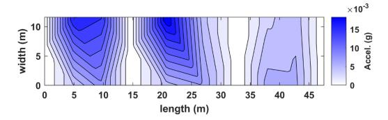
Figure B.75. Interpolated absolute-valued acceleration in plan view for truck pass 42 at the NOBL North bridge structure.
