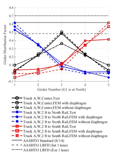
Figure C.401. GDF from negative strain near east side of pier, west direction loading.
