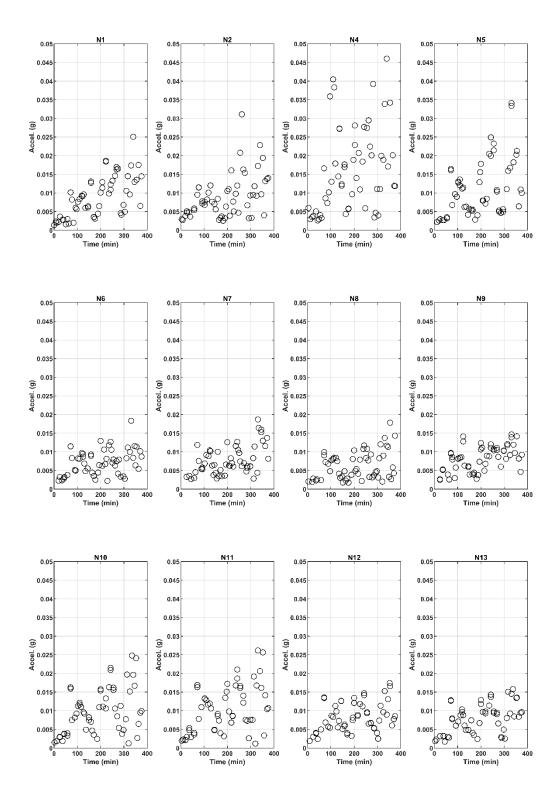
Figure 4.11. Absolute maximum acceleration values for each truck pass at the NOBL North.
