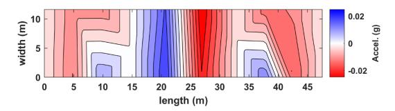
Figure B.26. Interpolated acceleration in plan view for truck pass 36 at the NOBL North bridge structure.
