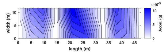
Figure B.56. Interpolated absolute-valued acceleration in plan view for truck pass 23 at the NOBL North bridge structure.
