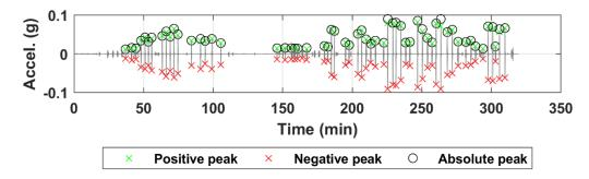
Figure B.98. Acceleration time history of sensor N07 for all truck passes at the NOBL East Yutan bridge structure.
