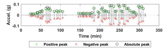
Figure B.104. Acceleration time history of sensor N13 for all truck passes at the NOBL East Yutan bridge structure.
