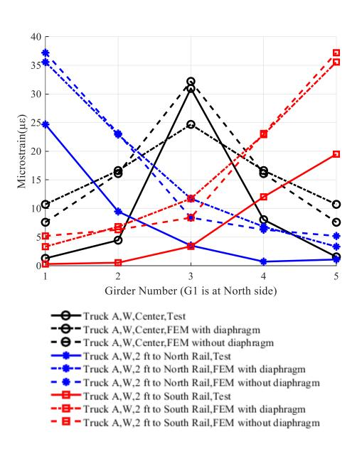
Figure C.398. Positive strain at 0.4 L of east end span, west direction loading
