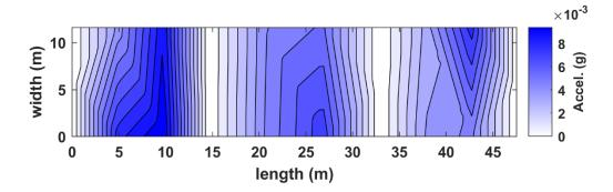
Figure B.78. Interpolated absolute-valued acceleration in plan view for truck pass 45 at the NOBL North bridge structure.
