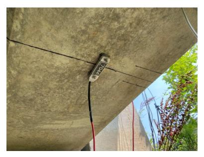
Figure 5.5. Strain transducer attached to the bottom flange of girder.
