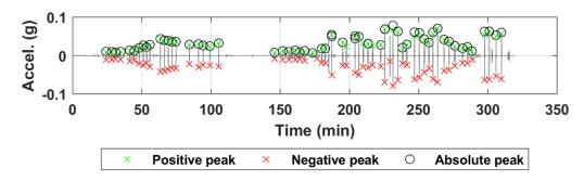
Figure B.109. Acceleration time history of sensor N18 for all truck passes at the NOBL East Yutan bridge structure.
