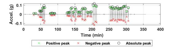
Figure B.235. Acceleration time history of sensor N01 for all truck passes at the NOBL West Yutan bridge structure.
