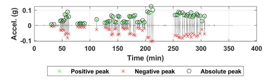
Figure B.239. Acceleration time history of sensor N06 for all truck passes at the NOBL West Yutan bridge structure.
