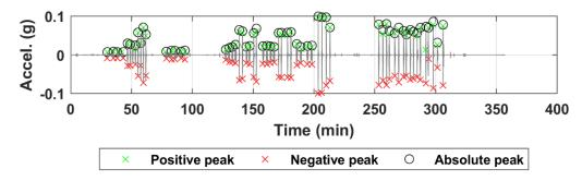
Figure B.236. Acceleration time history of sensor N02 for all truck passes at the NOBL West Yutan bridge structure.
