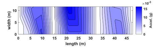
Figure B.51. Interpolated absolute-valued acceleration in plan view for truck pass 18 at the NOBL North bridge structure.
