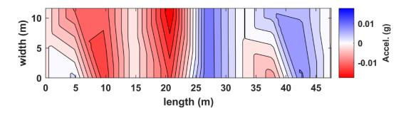
Figure B.8. Interpolated acceleration in plan view for truck pass 18 at the NOBL North bridge structure.
