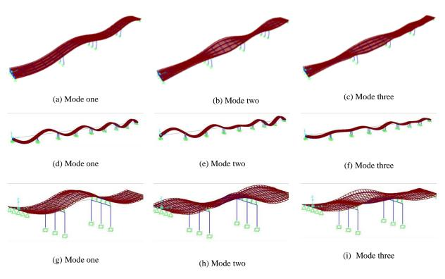
Figure 3.3. Mode shapes of the three selected bridges; (a), (b), (c) NOBL East steel bridge at Yutan; (d), (e), (f) NOBL West steel bridge at Yutan; (g), (h), (i) NOBL North concrete bridge in Omaha.
