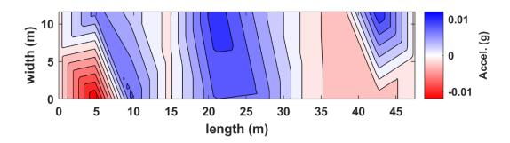
Figure B.36. Interpolated acceleration in plan view for truck pass 46 at the NOBL North bridge structure.
