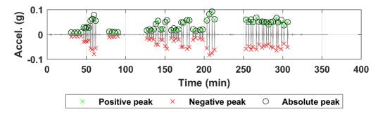
Figure B.246. Acceleration time history of sensor N13 for all truck passes at the NOBL West Yutan bridge structure.
