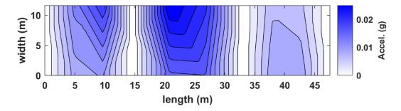
Figure B.72. Interpolated absolute-valued acceleration in plan view for truck pass 39 at the NOBL North bridge structure.
