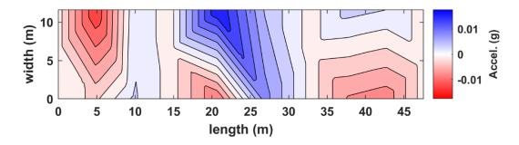
Figure B.14. Interpolated acceleration in plan view for truck pass 24 at the NOBL North bridge structure.
