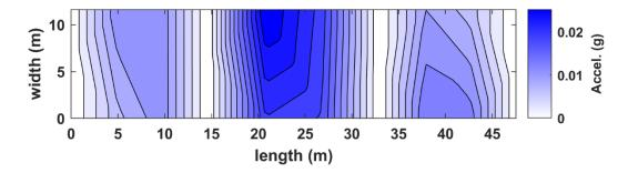
Figure B.70. Interpolated absolute-valued acceleration in plan view for truck pass 37 at the NOBL North bridge structure.
