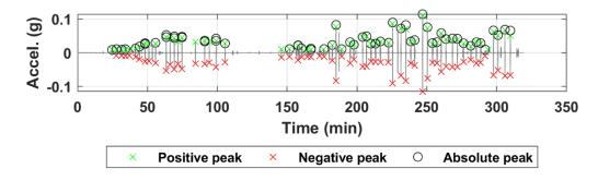
Figure B.94. Acceleration time history of sensor N02 for all truck passes at the NOBL East Yutan bridge structure.
