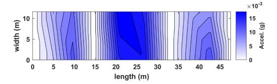
Figure B.63. Interpolated absolute-valued acceleration in plan view for truck pass 30 at the NOBL North bridge structure.
