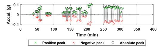
Figure B.240. Acceleration time history of sensor N07 for all truck passes at the NOBL West Yutan bridge structure.
