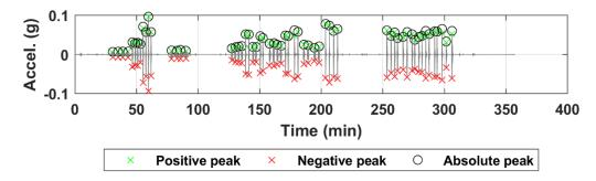
Figure B.243. Acceleration time history of sensor N10 for all truck passes at the NOBL West Yutan bridge structure.
