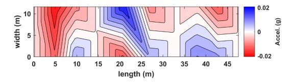
Figure B.24. Interpolated acceleration in plan view for truck pass 34 at the NOBL North bridge structure.
