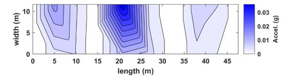
Figure B.76. Interpolated absolute-valued acceleration in plan view for truck pass 43 at the NOBL North bridge structure.
