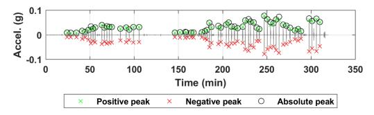
Figure B.112. Acceleration time history of sensor N21 for all truck passes at the NOBL East Yutan bridge structure.
