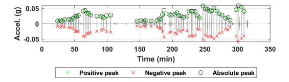
Figure B.111. Acceleration time history of sensor N20 for all truck passes at the NOBL East Yutan bridge structure.
