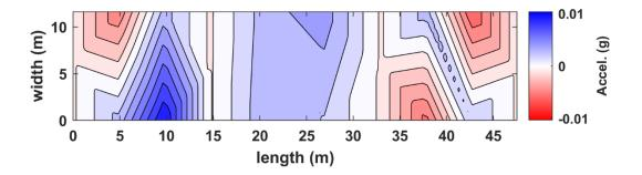
Figure B.34. Interpolated acceleration in plan view for truck pass 44 at the NOBL North bridge structure.
