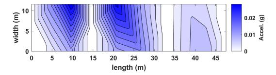
Figure B.73. Interpolated absolute-valued acceleration in plan view for truck pass 40 at the NOBL North bridge structure.
