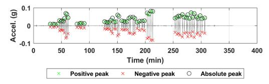
Figure B.254. Acceleration time history of sensor N21 for all truck passes at the NOBL West Yutan bridge structure.
