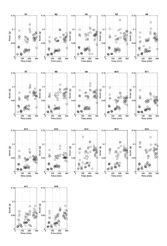
Figure B.234. Absolute maximum acceleration values for each truck pass at the NOBL West Yutan bridge structure.
