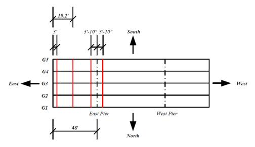
Figure 5.3. Strain transducers installation locations in the bridge.
