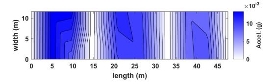
Figure B.90. Interpolated absolute-valued acceleration in plan view for truck pass 57 at the NOBL North bridge structure.
