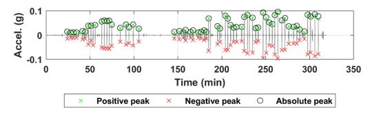
Figure B.106. Acceleration time history of sensor N15 for all truck passes at the NOBL East Yutan bridge structure.
