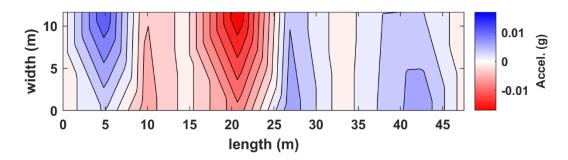
Figure B.15. Interpolated acceleration in plan view for truck pass 25 at the NOBL North bridge structure.
