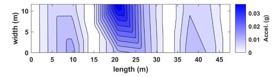
Figure B.49. Interpolated absolute-valued acceleration in plan view for truck pass 16 at the NOBL North bridge structure.
