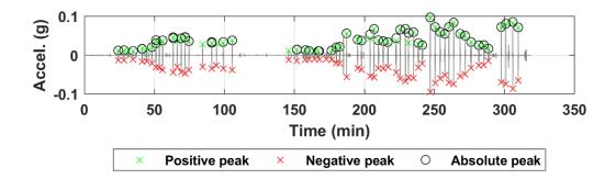
Figure B.108. Acceleration time history of sensor N17 for all truck passes at the NOBL East Yutan bridge structure.
