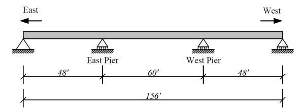
Figure C.374. Schematic elevation of bridge.
