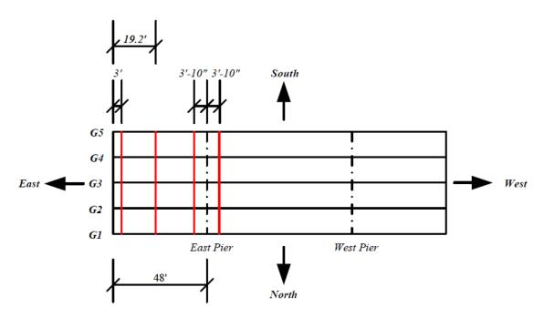
Figure C.376. Strain transducers installation locations in the bridge.
