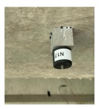
Figure 4.1. Example placement of a wired uniaxial accelerometer.
