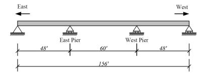
Figure 5.1. Schematic elevation of the bridge.
