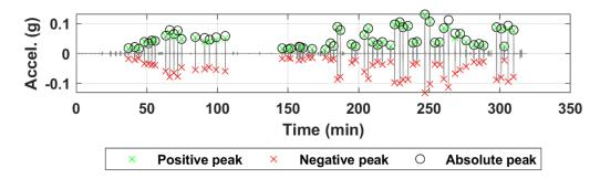
Figure B.95. Acceleration time history of sensor N04 for all truck passes at the NOBL East Yutan bridge structure.
