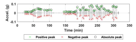
Figure B.100. Acceleration time history of sensor N09 for all truck passes at the NOBL East Yutan bridge structure.
