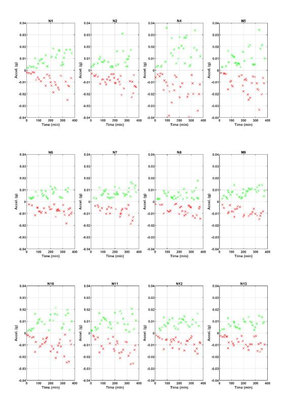
Figure 4.9. Maximum acceleration values for each truck pass at the NOBL North.
