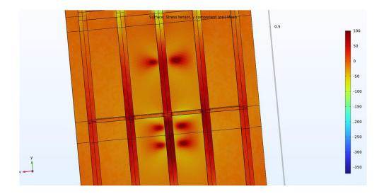
Figure C.395. COMSOL stress diagram for one truck at the center near the pier.
