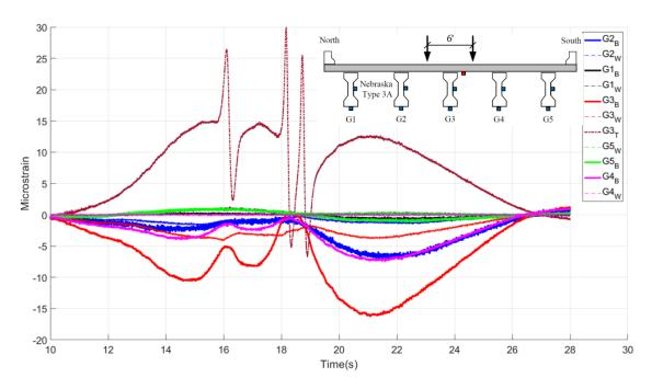
Figure C.394. Strain transducers results at east side of the pier for one truck A at the center from east to west.
