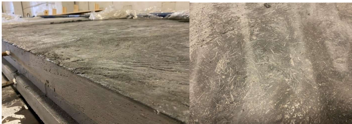
Figure 4.7: Specimen after stripping showing shear key (left) and fibers in the top surface (right)
