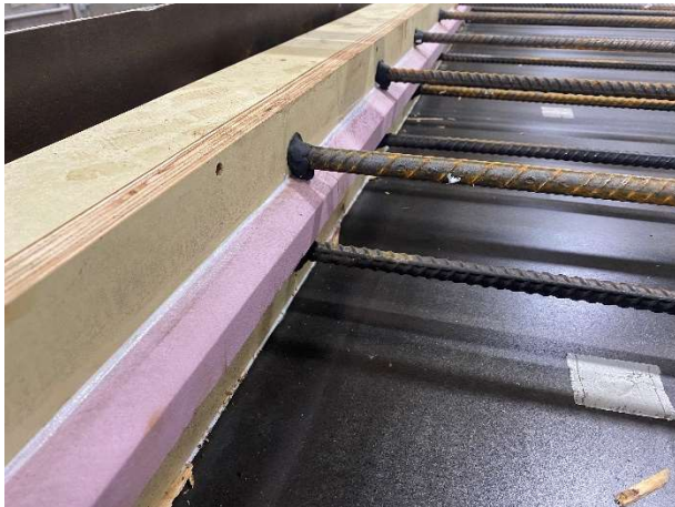
Figure 4.23: Forms for DIB specimen with solid slab
