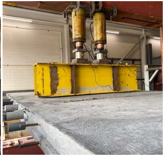
Figure 5.21: Vertical shear test setup and instrumentation
