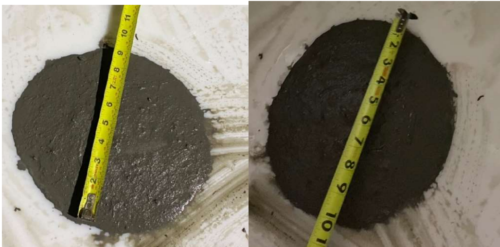
Figure 4.1: UHPC flow diameter of batch #1 (left) and batch #2 (right)
