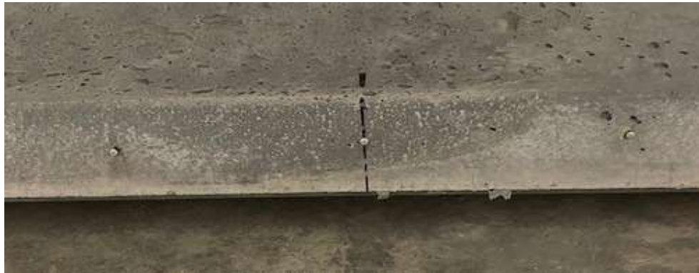
Figure 5.38: DEMEC gauges attached to bottom flange to measure strains due to post-tensioning
