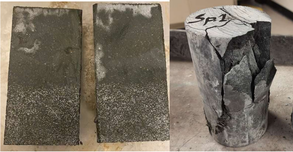
Figure 4.17: Saw cut cylinder showing severe fiber segregation (left) and failure mode (right)
