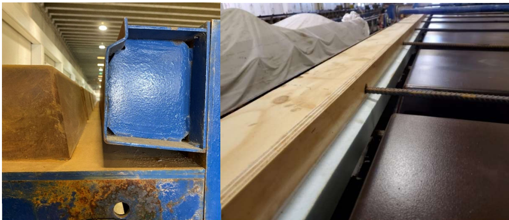
Figure 4.3: Forms and reinforcement of UHPC pretensioned specimen
