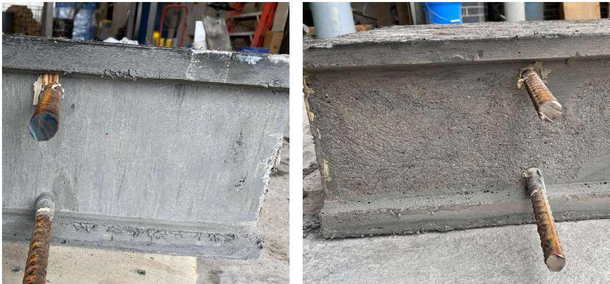
Figure 5.16: Finishing UHPC Shear key Surface: Smooth (left) and Sandblast (right)
