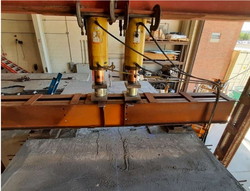
Figure 5.33: Longitudinal flexure cracks at the top of the solid slab
