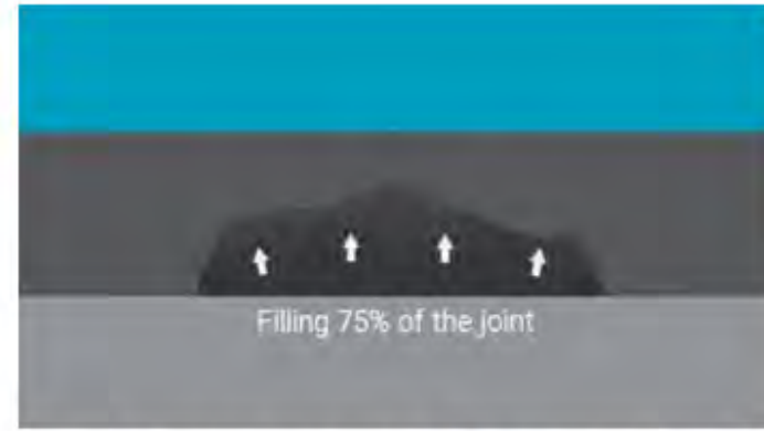
HMA softens VRAM, melts, filling voids in bottom part of the lift
