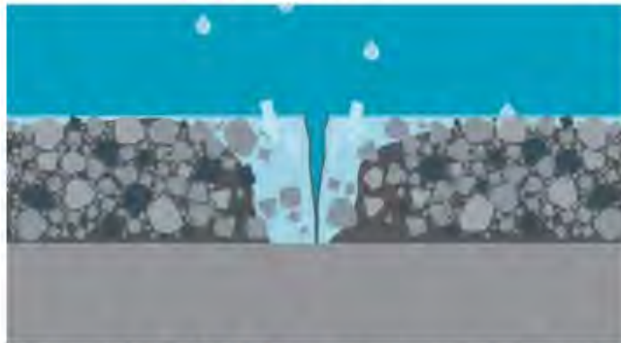
Without VRAM in a permeable mix, water over time damages the mix
