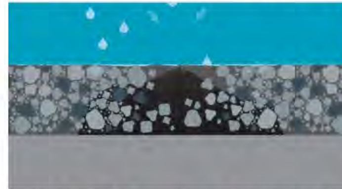
With VRAM, voids in lower portion of mix are sealed, protecting mix
