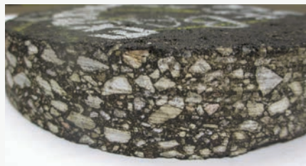
Core sample of new SLX mix used on US-77 – Lincoln South.
