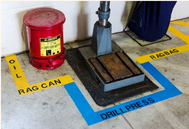
The Stapleton maintenance yard staff has worked “Five S” methodology into their shop’s layout, including clearly labeled items.
