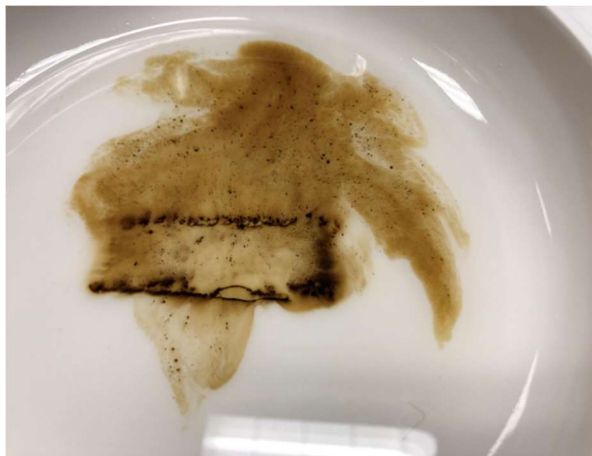
Figure 14 - The 5-min soak of Product 5 left solids in solution.
