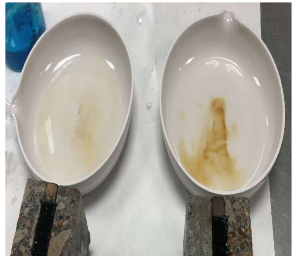
Figure 10 - Product 3, 1-min. and 5-min. post-test dishes showing discoloration.
