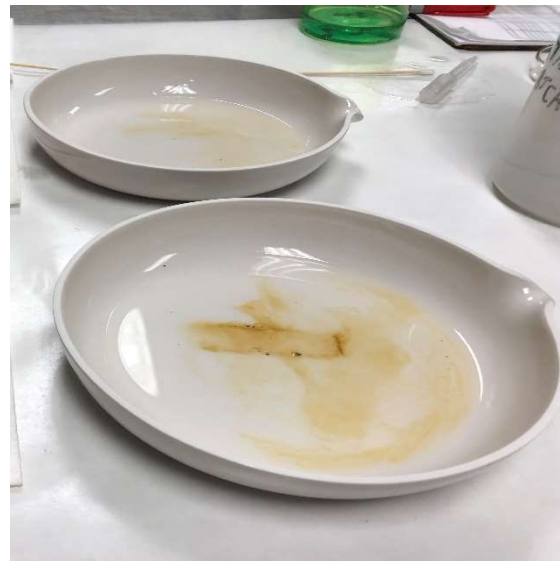
Figure 7- The Product 1 field sample 1-minute soaking dish (top) and the 5-minute soaking dish (bottom) each showed discoloration of the penetrating concrete sealer. The 5-minute soak shows more dissolution than the 1-minute soak.
