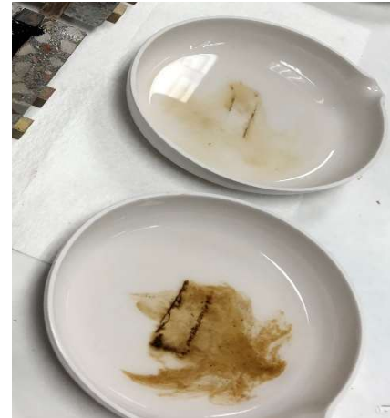
Figure 13 - Product 5; the 5-min (bottom dish) soak showed the most discoloration of any of the tests.
