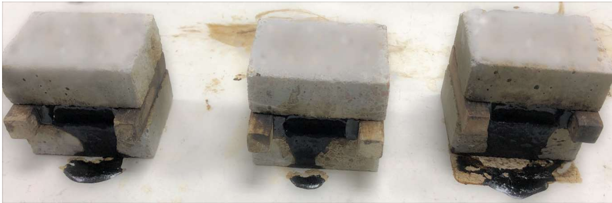
Figure 16 - Hot pour sealant flowed out of the cupped blocks after being ponded with Product 5.
