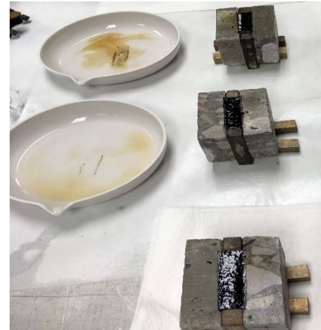
Figure 12 - Discoloration from the Product 4 testing was more intense than in Products 1, 2, and 3. The 5-min dish (top) also shows some solids falling off the block.
