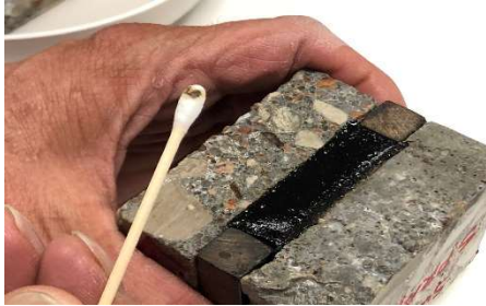
Figure 6 - The sprayed block was swabbed at the interfacial bond. The swab shows discoloration occurred after spraying.
