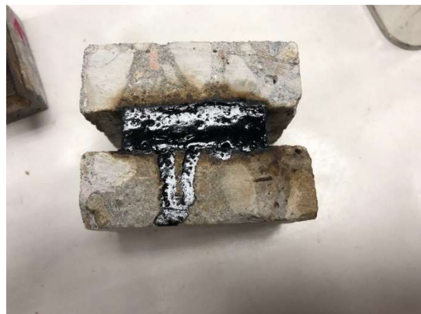
Figure 15 – NE-3405 sealant ran down the face of Product 5's 5-minute block.
