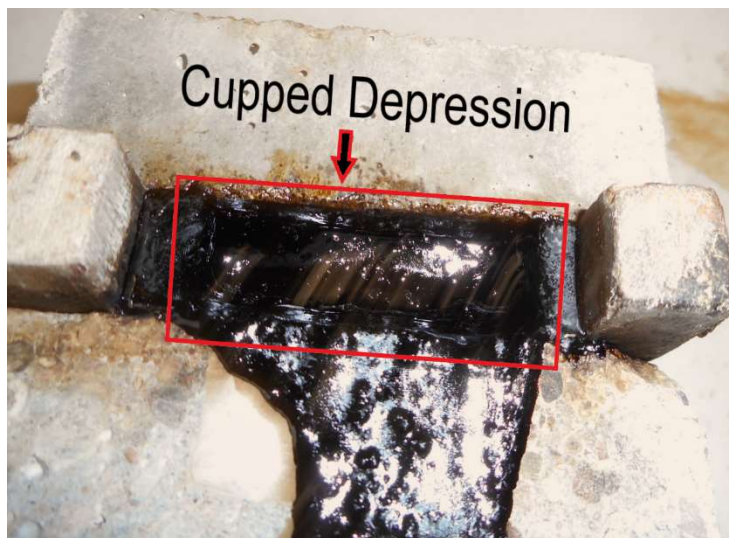
Figure 5 - A set of blocks was modified to create a cupped depression in the hot-pour sealant.
