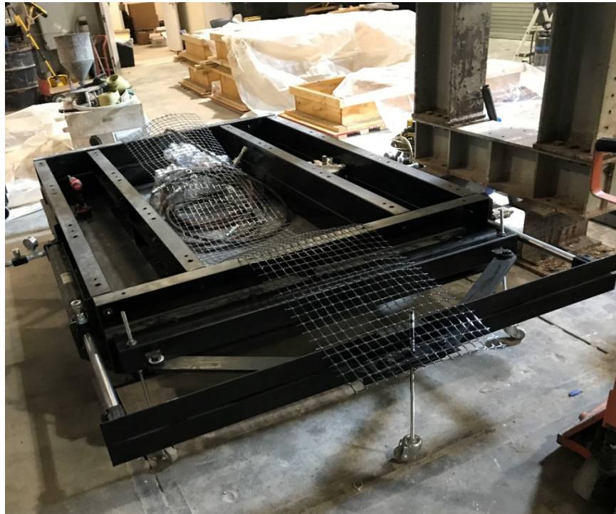
Figure 4.6 A modified large-scale pull-out test box for the testing of soil-geosynthetic interactions.
