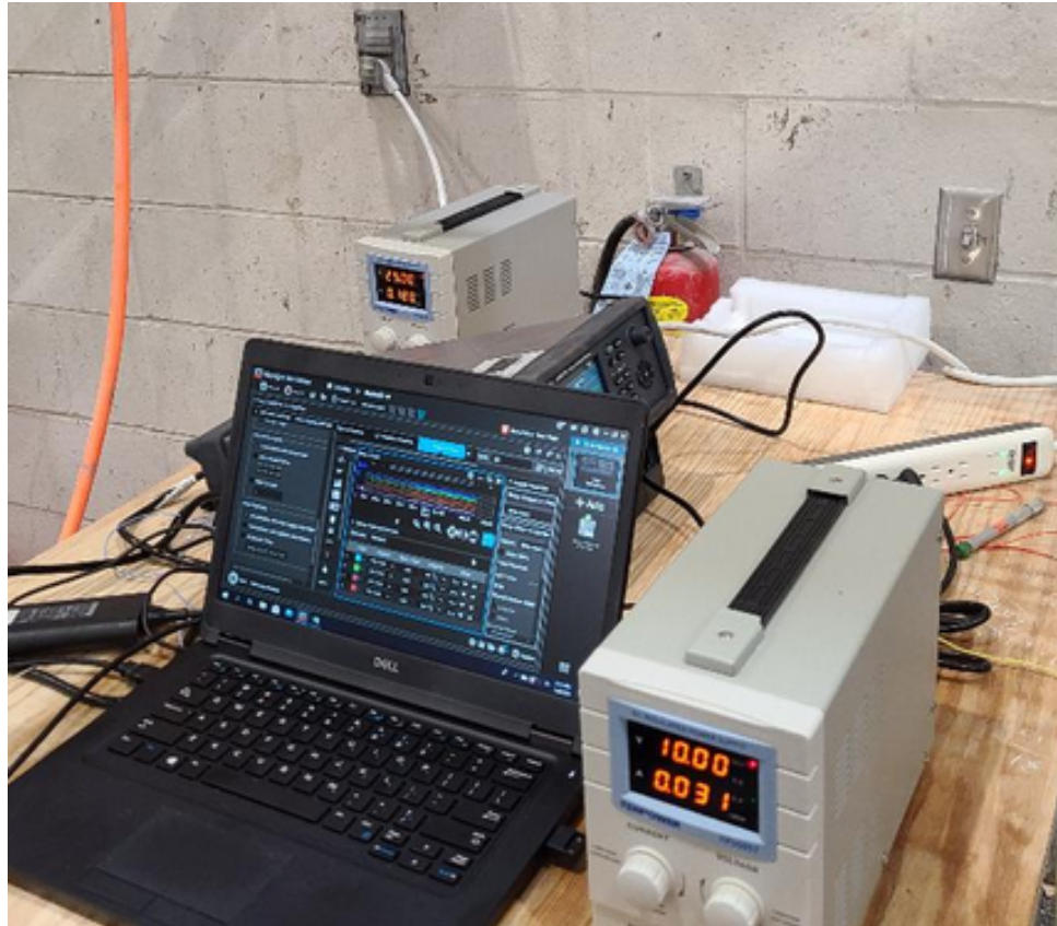
Figure 4.14 The data acquisition system used to automatically obtain the monitoring data during the pullout tests.
