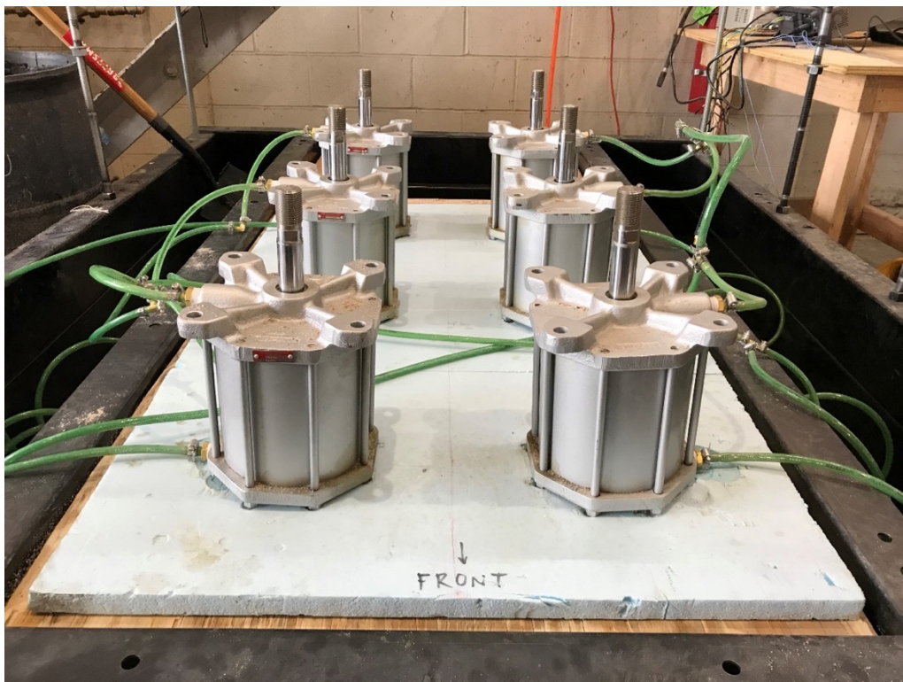
Figure 4.10 The pneumatic pistons used to apply the vertical pressure to the soil.
