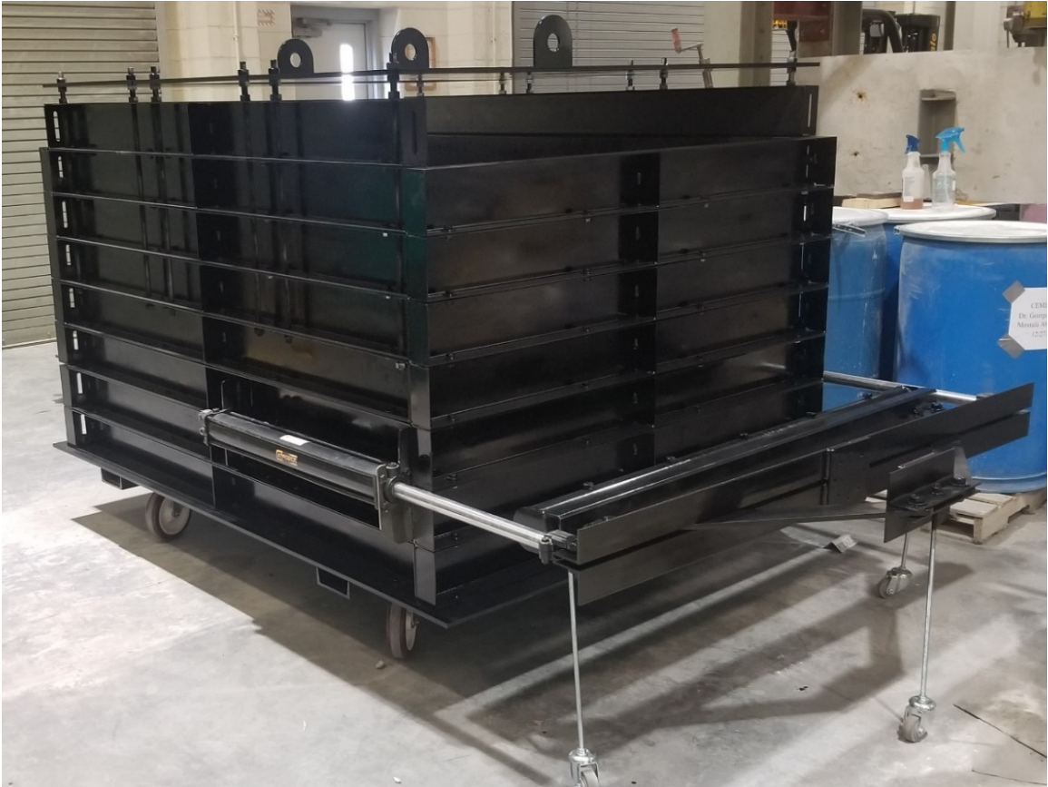
Figure 4.5 A photo of the fully assembled large-scale pullout test box by the research team.
