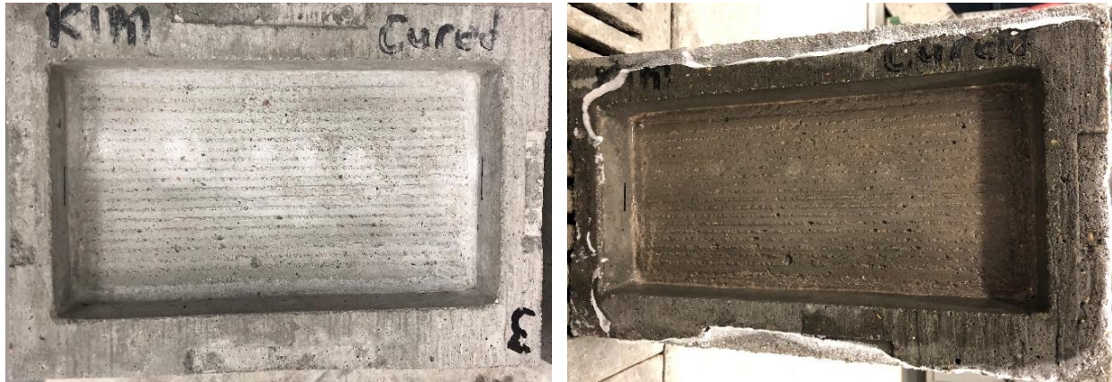
Figure 10 - B3 before testing (left) and after 85 F-T cycles showed moderate-heavy scaling on the rim and outer surfaces of the block.
