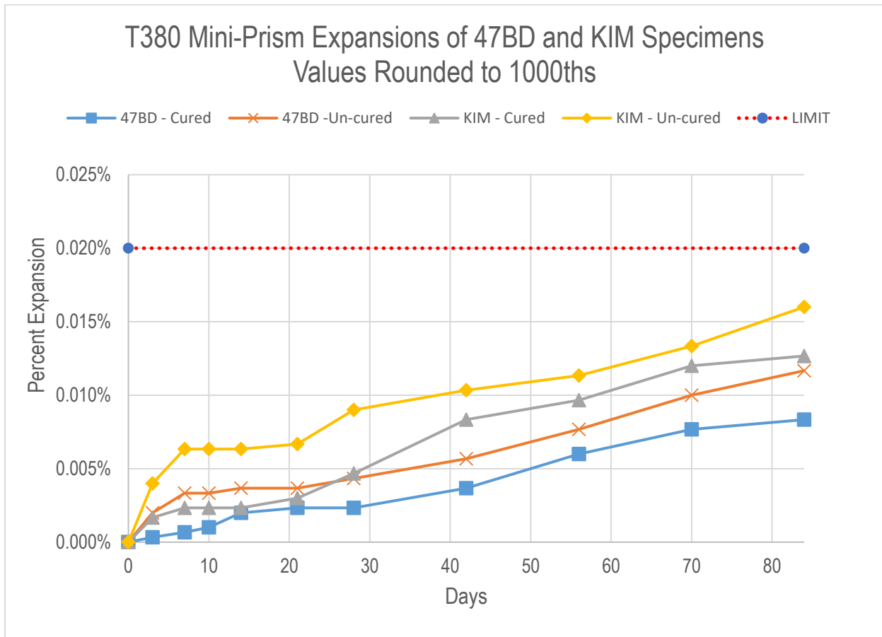
Figure 20 - T380 expansions comparing 47BD and KIM mixed specimens.
