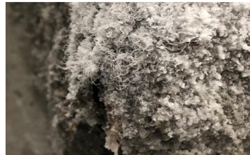
Figure 18 - Long, hair-like crystals formed on B7.
