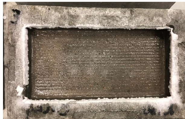
Figure 11 - NaCl deposited on the rim and outer surfaces of the ponding block during F-T testing.
