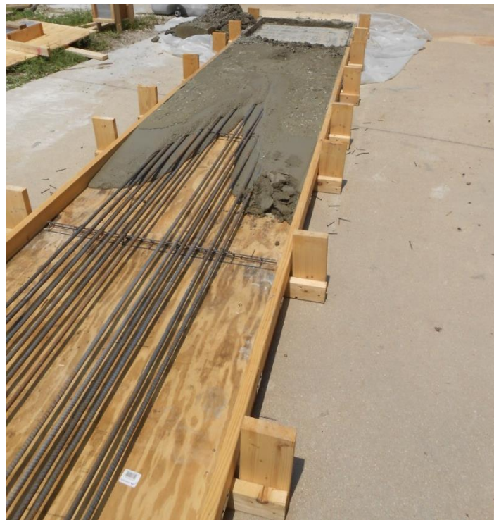
Figure 2.6 – Photo of concrete flow in the field test No. 2 (sudden loss of workability)
