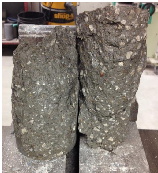
Figure 3.8 – Coarse aggregate distribution in hardened concrete (HVSI = 0)
