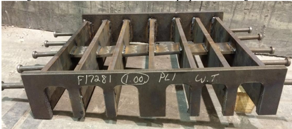
Figure 5.3: Photo of the anchorage block after assembly and before installation
