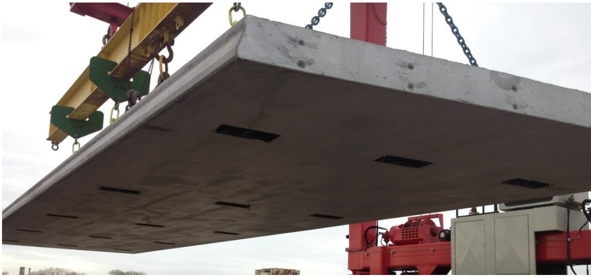
Figure 2.17 – Photo of full size demonstration deck panel showing panel soffit and shear pockets
