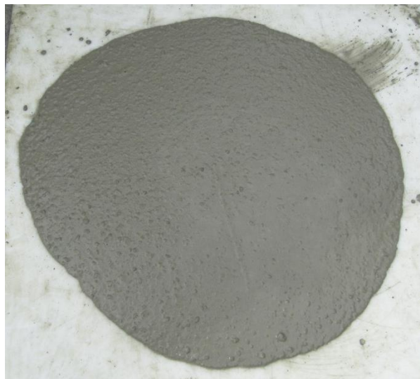
Figure 2.23 – Slump flow of the SCC mixture used in the pumping test (VSI = 0)
