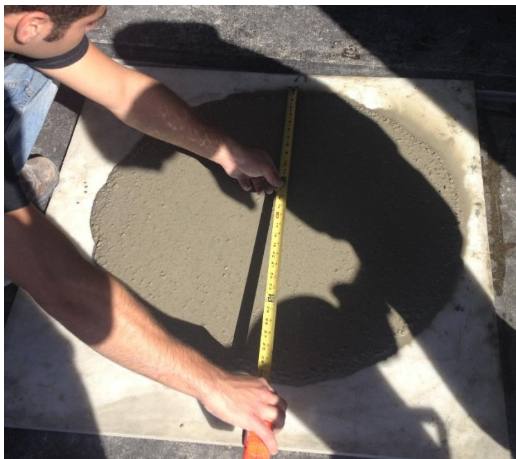
Figure 2.21 – Slump flow of the SCC mixture used in filling transverse joints (VSI = 1.0)
