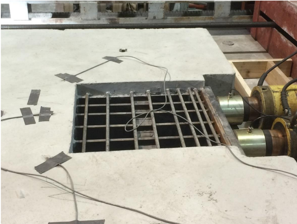
Figure 5.15: Photo of the anchorage zone when loaded at 600 kips
