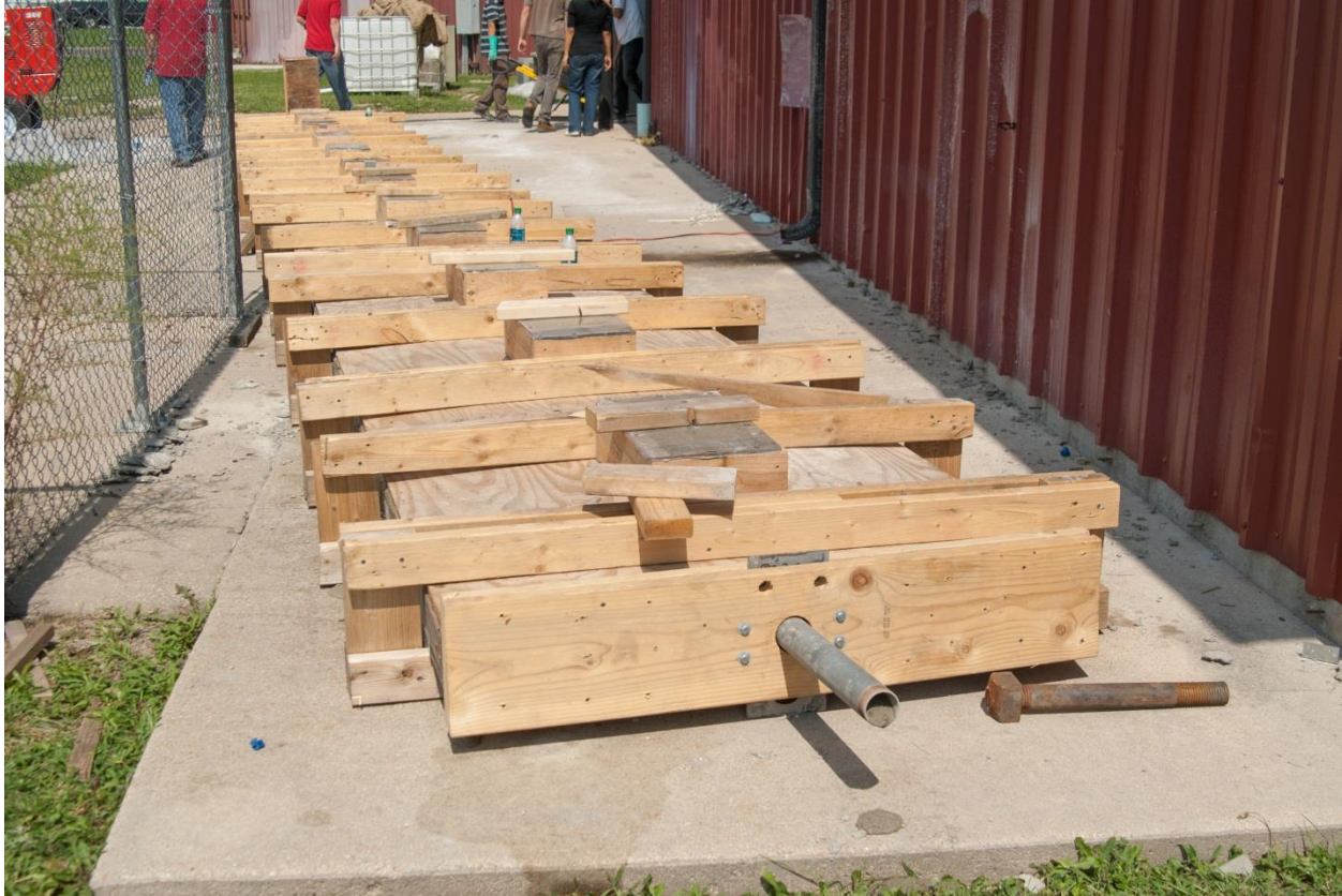
Figure 2.13 – Photo after the completion of casting from both ends
