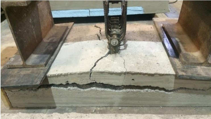
Figure 4.6: Test setup and failure mode of first specimen
