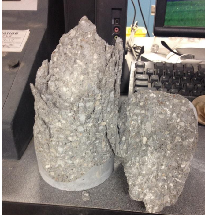
Figure 2.22 – Coarse aggregate distribution in joint concrete (HVSI = 1)
