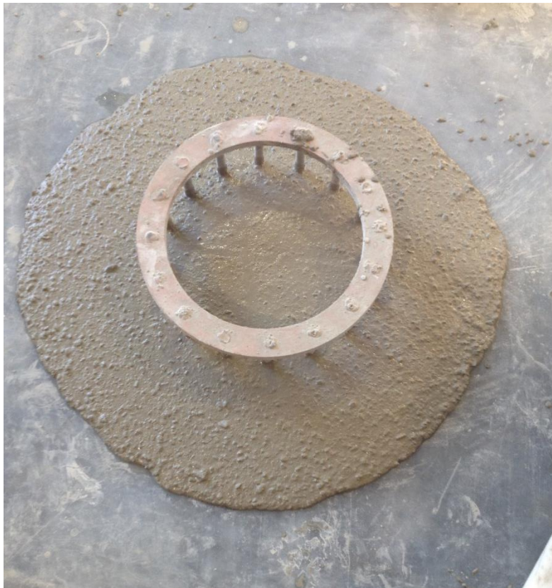
Figure 3.3 – Slump flow (top) and J-ring (bottom) tests (VSI = 0)
