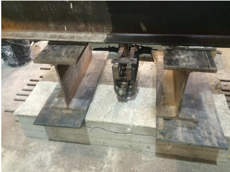
Figure 4.6: Test setup and failure mode of first specimen
