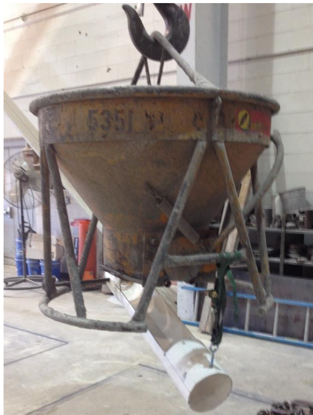
Figure 3.5 – The bucket and chute used in pouring SCC
