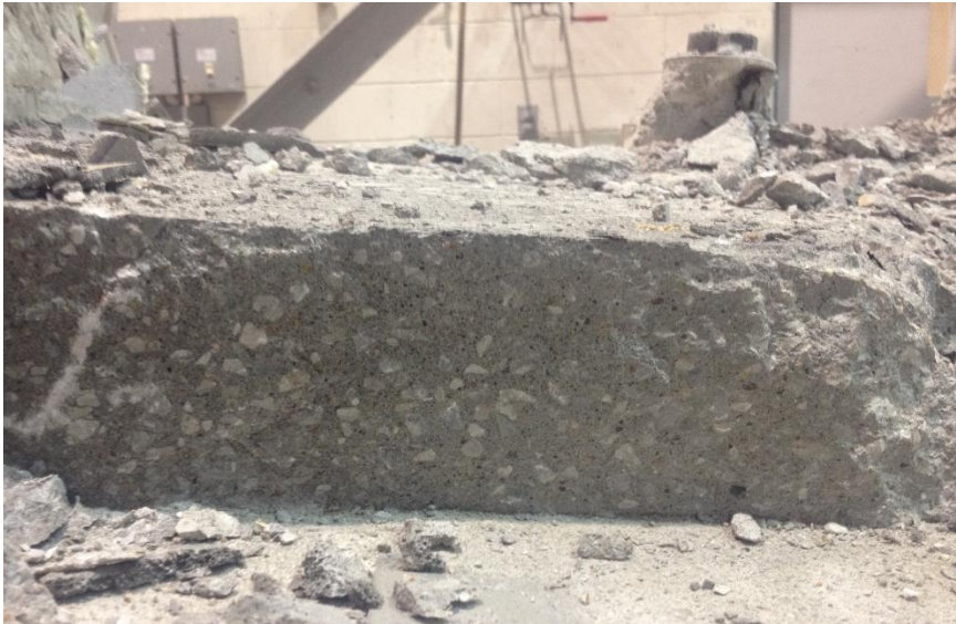
Figure 2.29 – Coarse aggregate distribution in haunch concrete (HVSI = 1.0)
