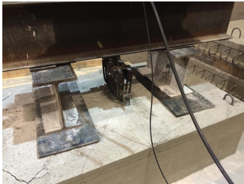
Figure 4.15: Failure mode of the second deviator
