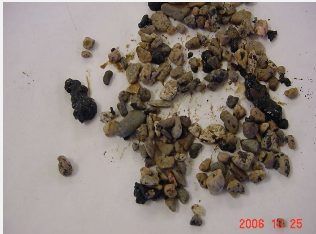
Dirty Natural Aggregate (2.2% #200) – with HFMS-2P Emulsion
