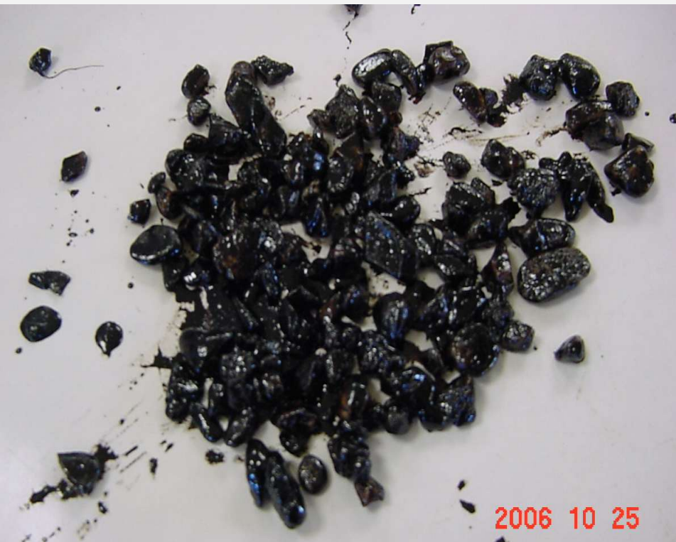
Washed Natural Aggregate – with CRS-2P Emulsion
