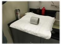
Figure 19 shows the surface drying of a previously submerged core before the measuring the final mass.
