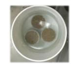
Figure 6 shows cores submerged in water.
