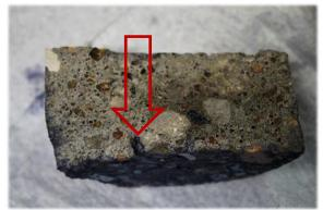
Figure 7 shows the control core. Slight blue dye can be seen penetrating at the surface.
