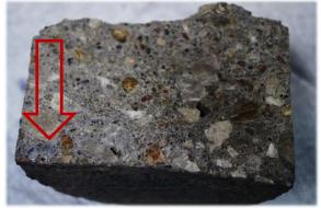
Figure 10 shows the Product 3 core. Slight blue shading can be seen in the left corner, caused by a chip in the surface.
