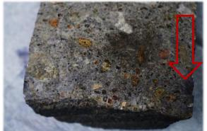
Figure 9 shows the Product 2 core. Blue shading can be seen across the middle.
