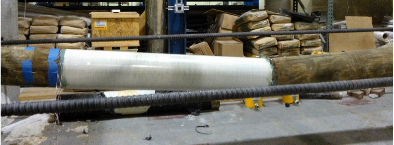
Figure 5.9: Failure of specimen 3 (2 inch deep damage filled with grout)
