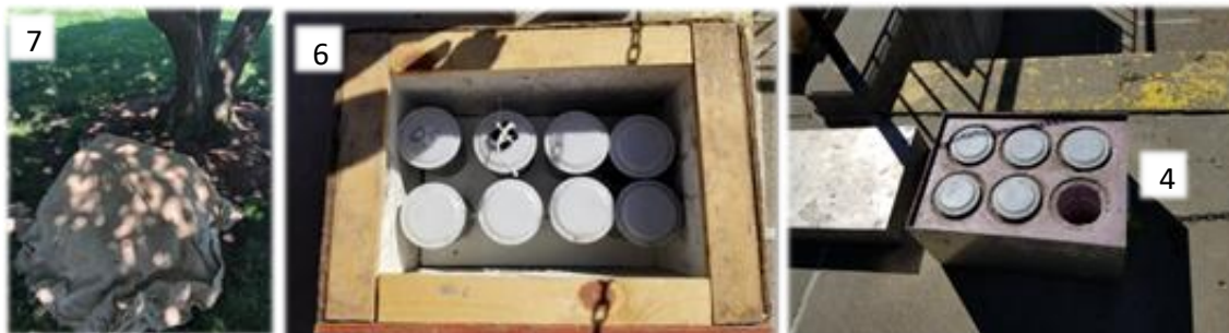
Figure 6- Hot Weather Curing Methods
