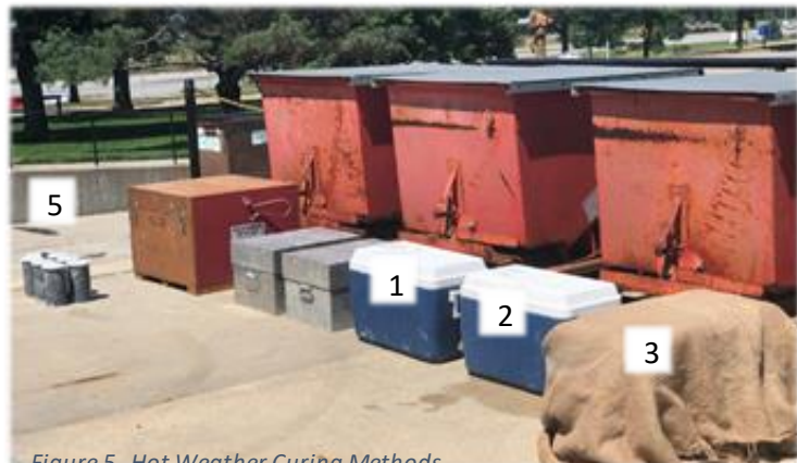
Figure 5- Hot Weather Curing Methods
