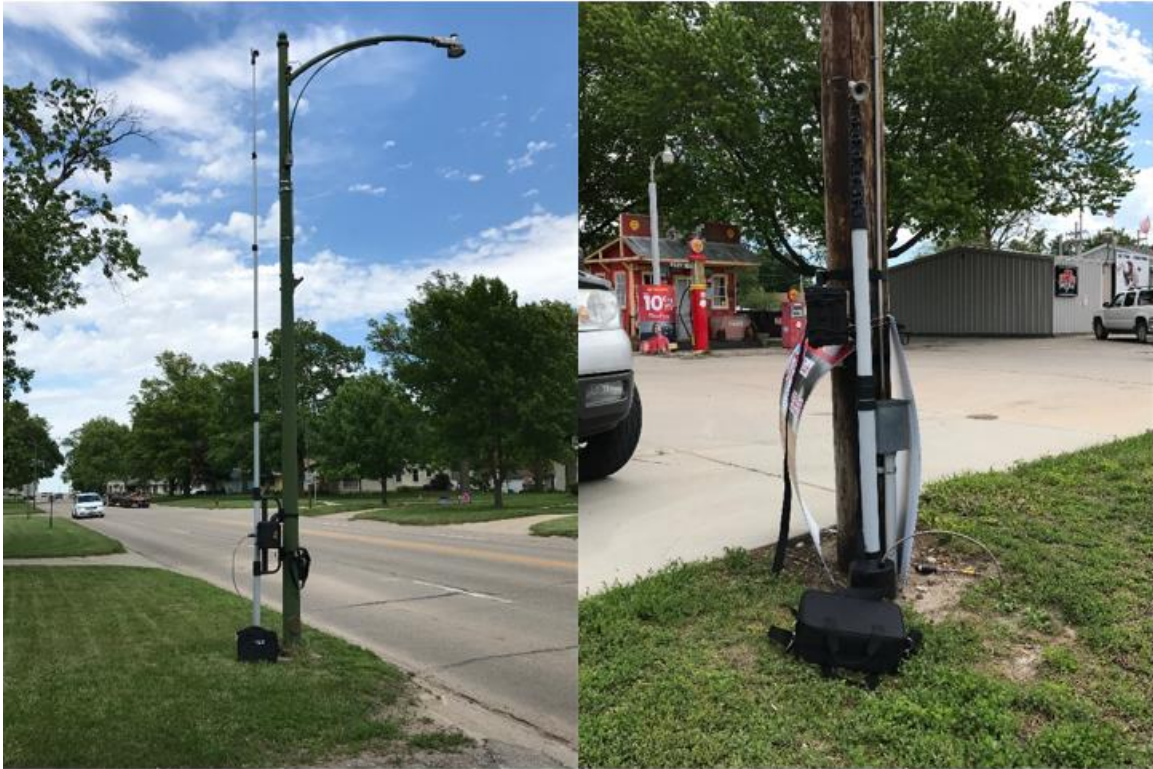
Figure 3.1 Setup of MioVision Scout cameras
