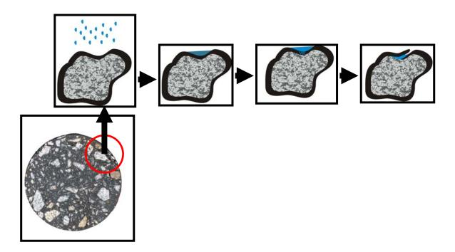
Figure 1.1 Illustration of Moisture Damage Mechanisms
