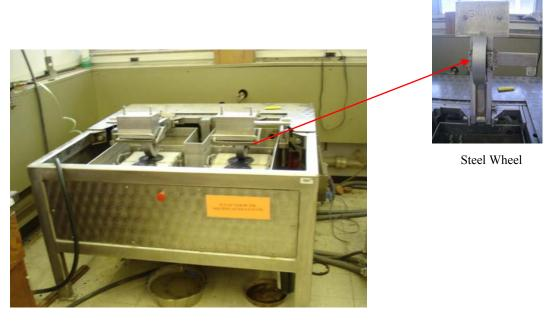
Figure 3.8 Hamburg Wheel-Tracking Device
