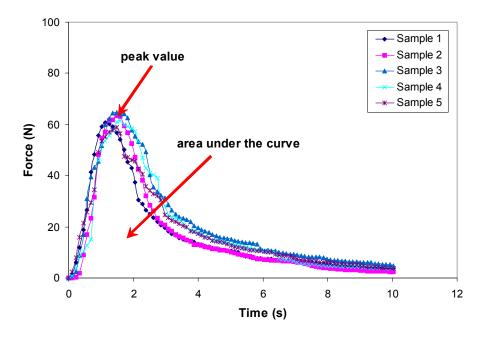
Figure 3.13 Testing Results of Five Asphalt Binder Replicates
