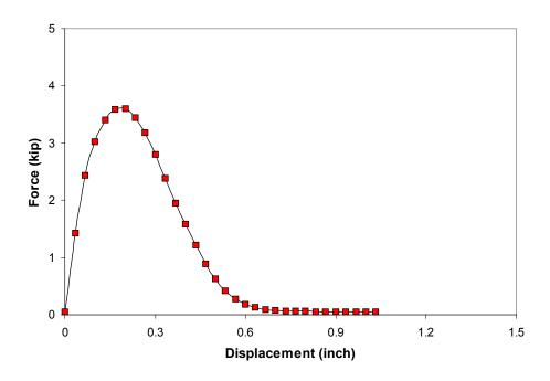
Figure 3.5 Typical AASHTO T-283 Testing Result
