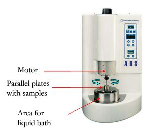
Figure 3.10 Dynamic Shear Rheometer
