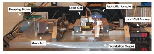
**Figure 3.11** Fracture-Damage Testing Device Set-up (Freitas *et al.* 2006)
