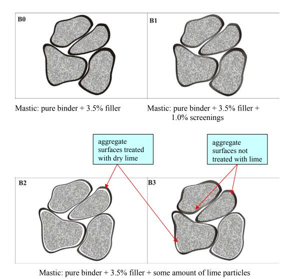
Figure 4.11 Illustrations Representing Mastic-Aggregate System of Each Mix
