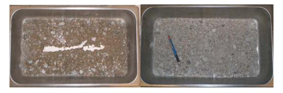
Figure 4.9 Lime Slurry Treated Aggregates (Before and After Oven Dry)
