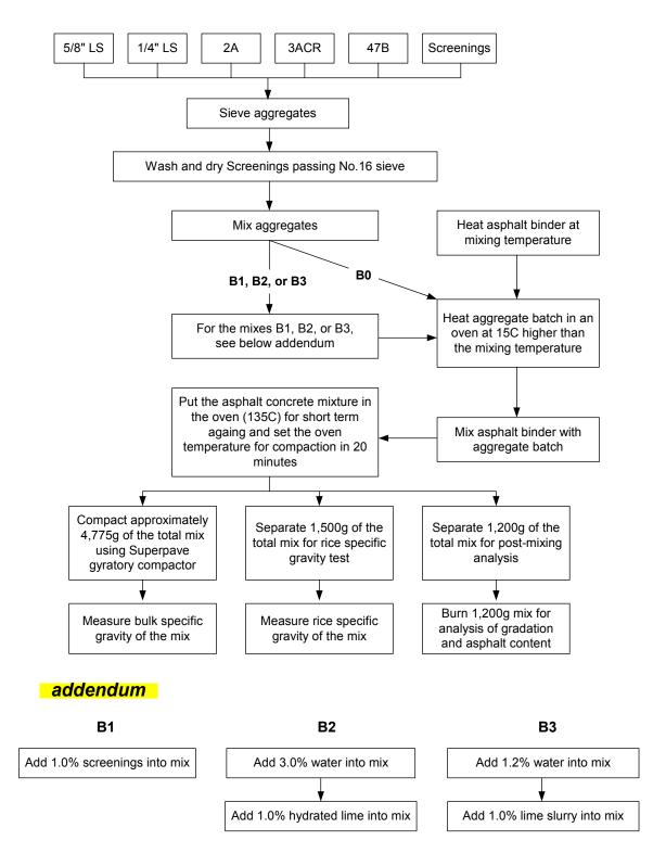
Figure 3.3 Mix Design Procedure
