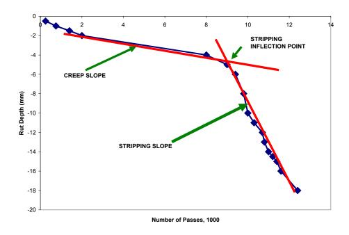
Figure 3.9 Typical Hamburg Testing Results
