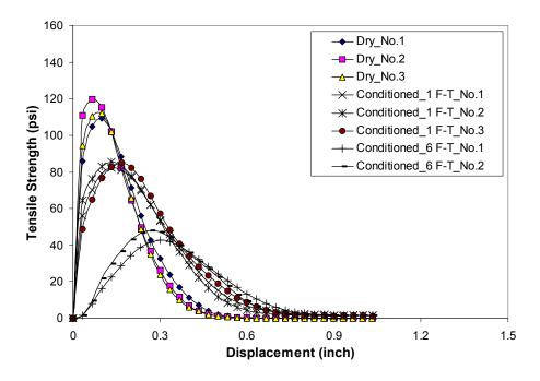
Figure 4.1 AASHTO T-283 Testing Results (B3 Mix)
