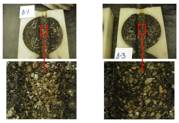
Figure 4.4 Stripping Observed After APA Testing (B1 vs. B3)
