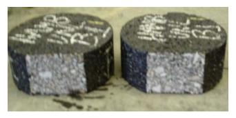
Figure 4.5 Hamburg Specimens After Being Cut
