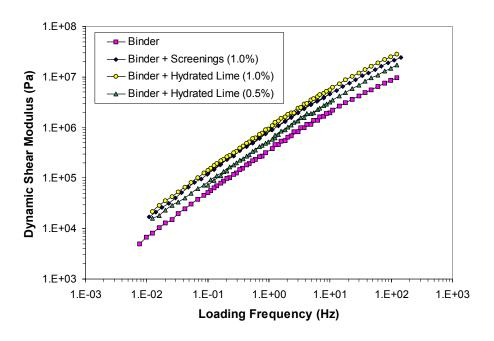
Figure 4.12 Master Curves at 30°C of Each Binder/Mastic
