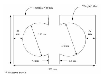
Figure 3.7 Hamburg Testing Mold
