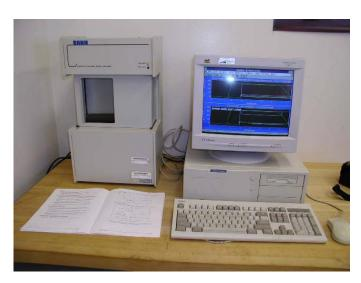
Figure 3.14 Wilhelmy Plate Testing Device
