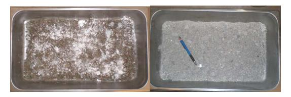
Figure 4.8 Dry Lime Treated Aggregates (Before and After Oven Dry)
