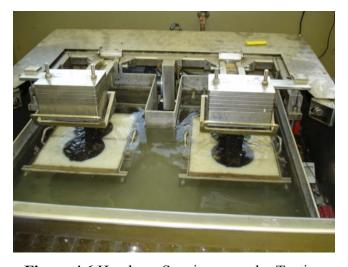
Figure 4.6 Hamburg Specimens under Testing
