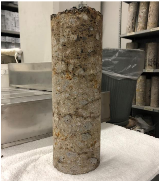
Figure 4. Wet & Dry Core Sample after 18 months
