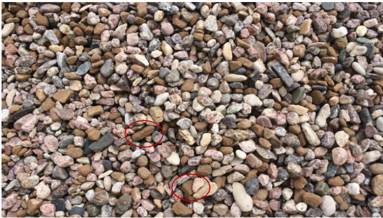
Figure 1. The red circle shows the lightweight aggregate pieces observed throughout the stockpile.
