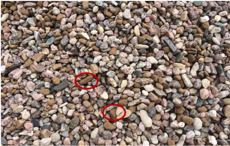
Figure 1: The red circle shows the lightweight aggregate pieces observed throughout the stockpile.
