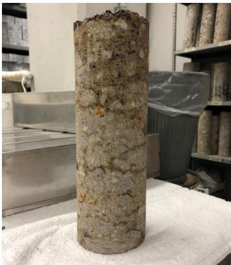
Figure 4. Wet & Dry Core Sample after 18 months
