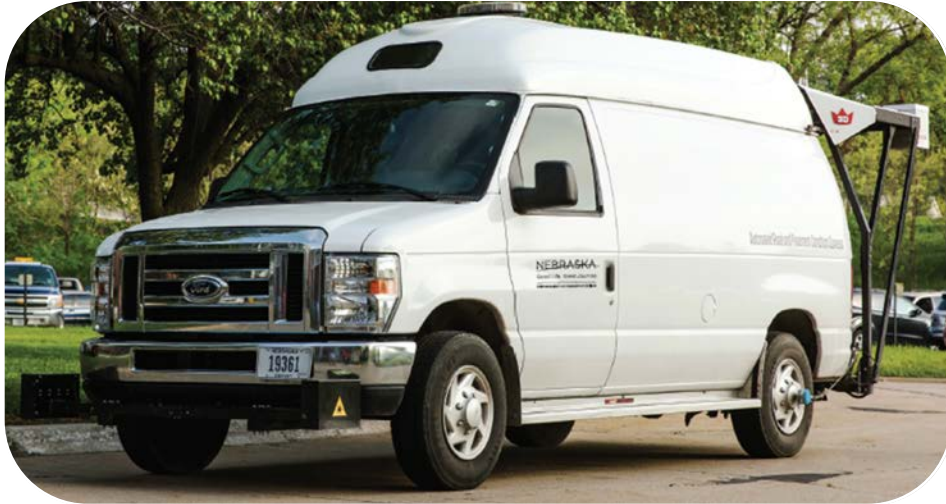
Automated Data Collection (Rutting, Faulting, IRI, 3D Surface, Photos, & GPS data)
