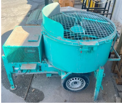
Figure 4.20 UHPC high shear mixer at UNL (Imer 750)
