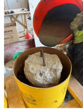
Figure 4.21 Formwork and casting of UHPC jacket
