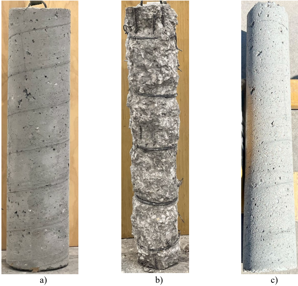
Figure 4.15 Surface preparation of columns a) original column, b) column after cover removal, and c) column after surface sand blasting.
