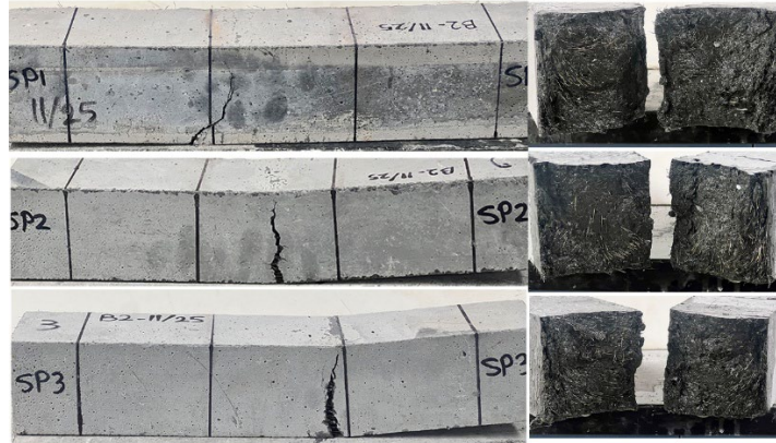
Figure 4.8 Tested flexural prisms after failure.
