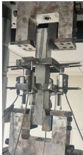
Figure 4.9 Direct tension testing of UHPC prism
