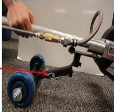
(a) 2 nd Generation : foldable wheel assembly
