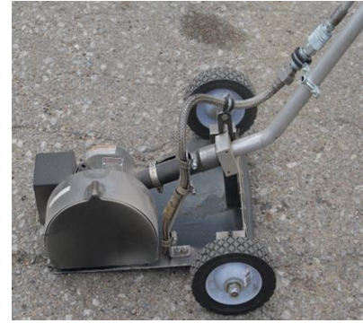
(b) 3 rd Generation : Larger, more stable structure with larger rubber foam wheels
